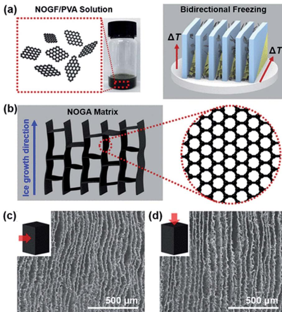
Fig. 10 Schematic of the synthesis of aerographene by bidirectional freezing (a), aerographene structure (b) and aerographene SEM images (c and d).<sup>176</sup> Reprinted with permission from ref. 176 (Copyright © 2018, American Chemical Society).
