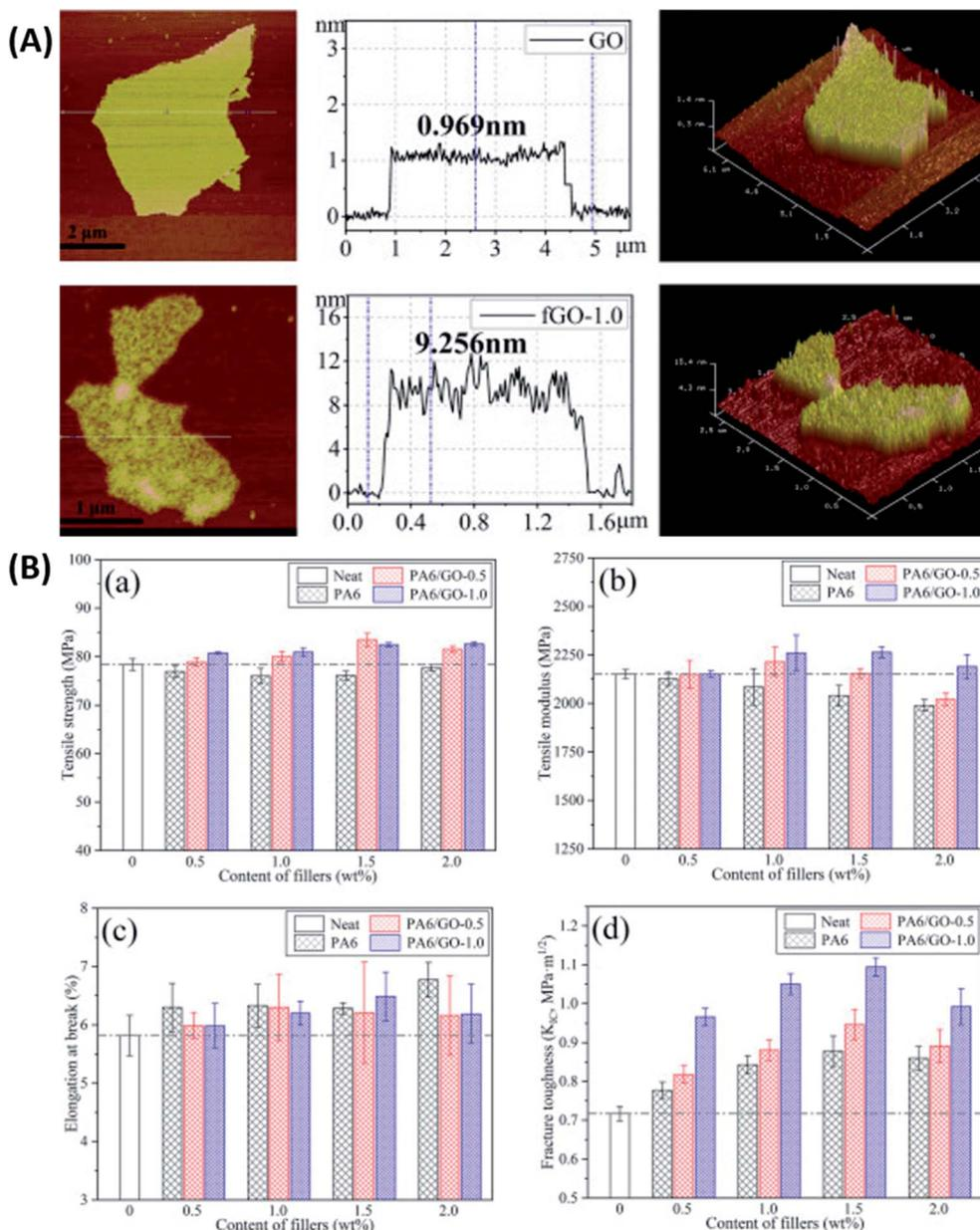
Fig. 7 (A) AFM images and sheet thickness analysis of GO (a) and PA6-GO (b) and (B) tensile (a-c) and fracture (d) properties of epoxy composite.<sup>128</sup> Reprinted with permission from ref. 128 (Copyright © 2018 Elsevier Ltd).
