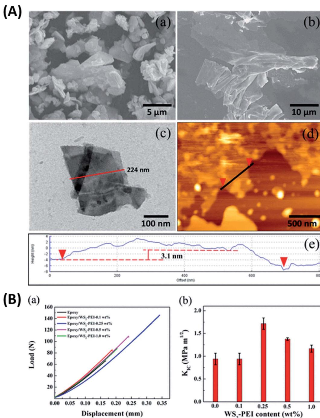
Fig. 8 (A) SEM images of bulk WS<sub>2</sub> (a), SEM (b), TEM (c) and AFM (d and e) images of PEI functionalized WS<sub>2</sub> and (B) fracture toughness of the PEI-WS<sub>2</sub>/epoxy composites (a and b).<sup>8</sup> Reprinted with permission from ref. 8 (Copyright © 2017, American Chemical Society).
