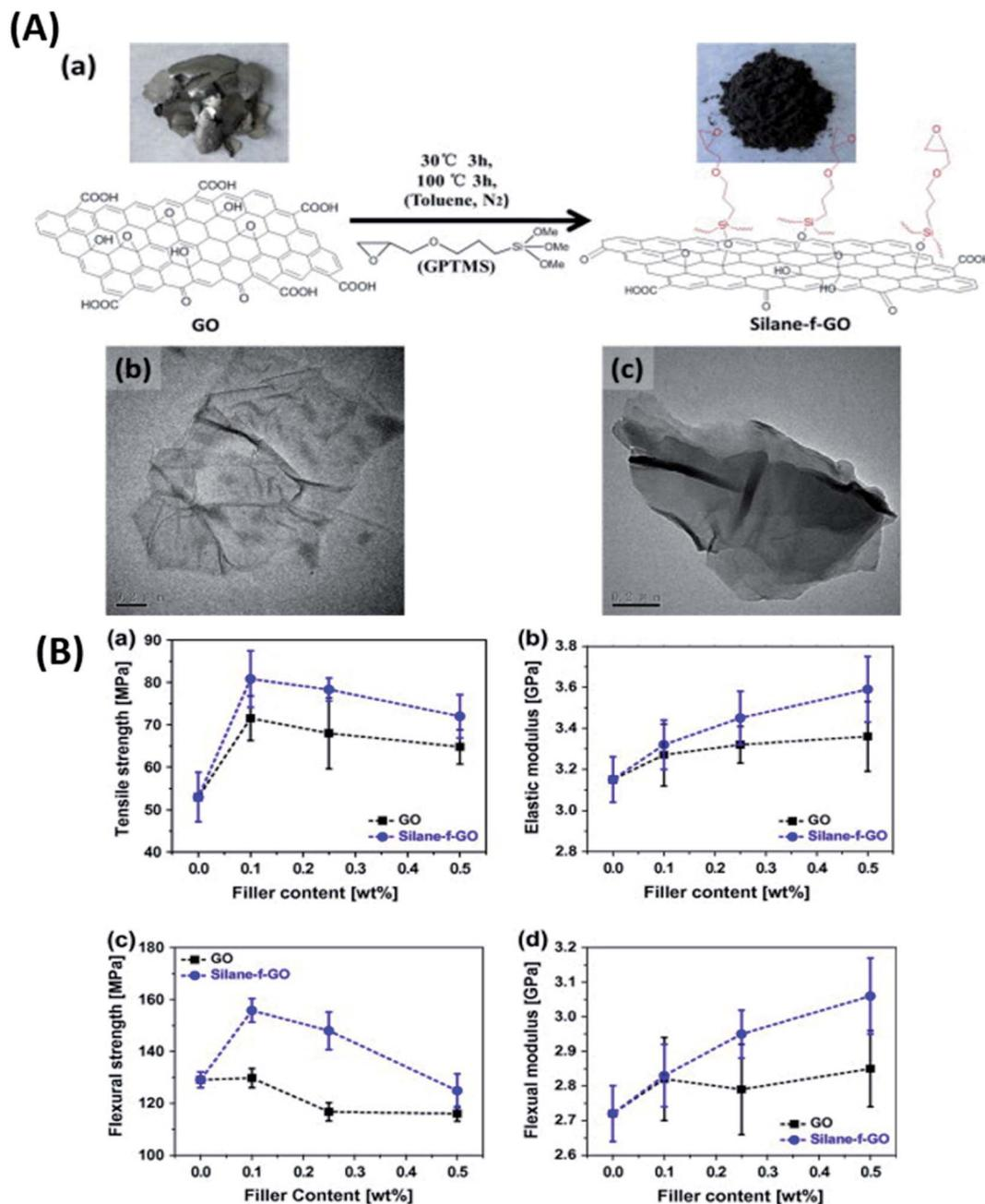
Fig. 6 (A) Synthesis route schematic of silane functionalized GO (a) and TEM images of GO (b) and silane-f-GO (c) and (B) mechanical properties of epoxy nanocomposites (a–d).<sup>66</sup> Reprinted with permission from ref. 66 (Copyright © 2014 Elsevier Ltd).
