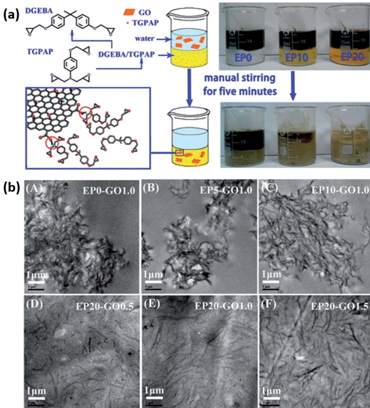
Fig. 4 Schematic and digital images of composites fabricated by the phase transfer method (a); TEM images of nanocomposites at various concentrations of the filler (b).<sup>110</sup> Reprinted with permission from ref. 110 (Copyright © 2016, American Chemical Society).
