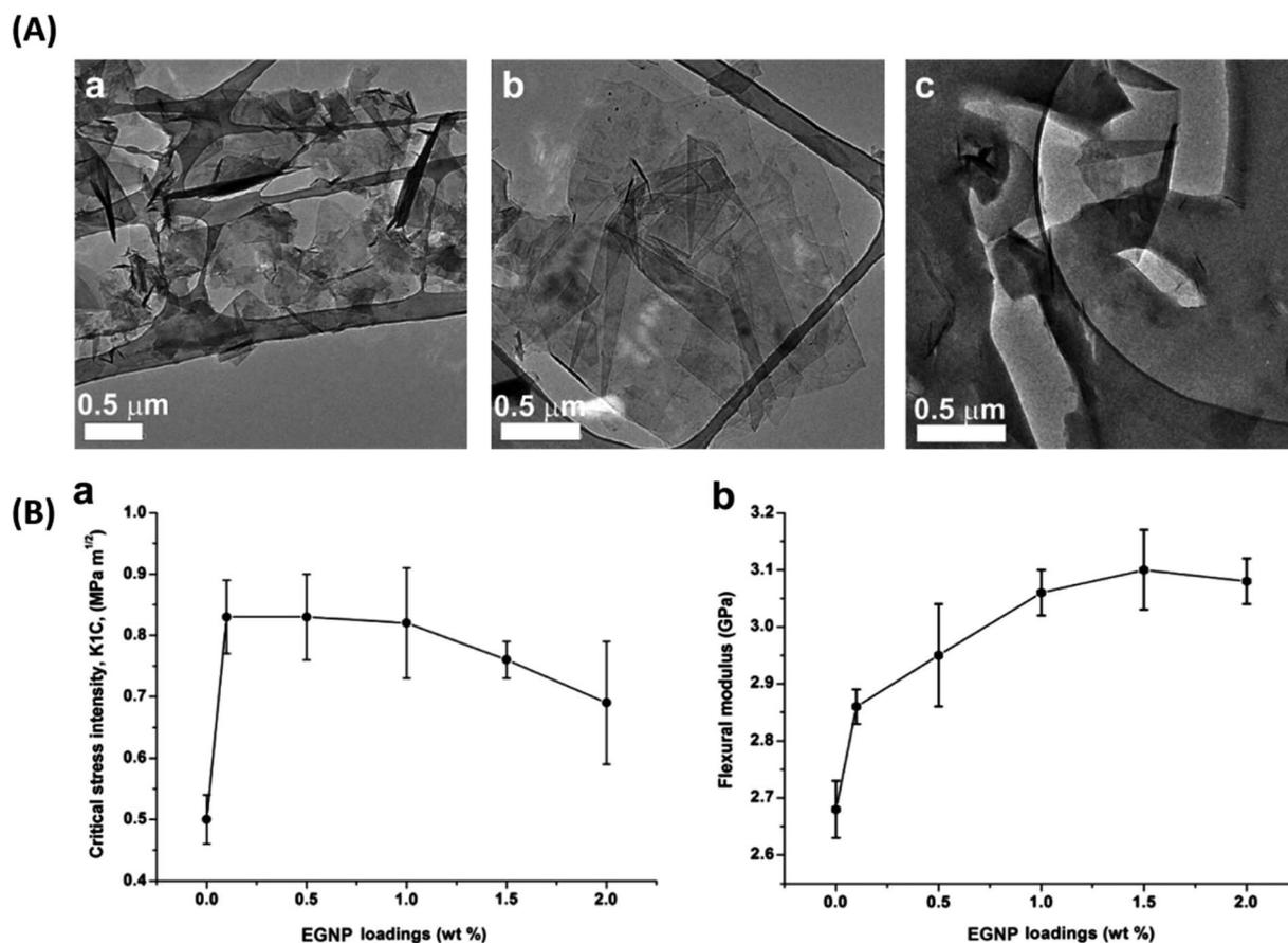
Fig. 5 (A) TEM images of amine-EGNPs (a and b) and 0.5 wt% amine-EGNP/epoxy composite (c). (B) Mechanical properties of epoxy composites with different EGNP loadings.<sup>65</sup> Reprinted with permission from ref. 65 (Copyright © 2012 Elsevier B.V.).
