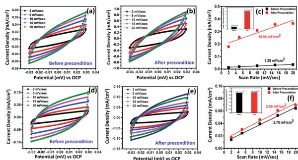
Fig. 3 CV curves recorded at different scan rates to estimate the double layer capacitance ( $C_{\text{dl}}$ ) for (a and b)  $\text{Ni}_{2.5}\text{Co}_5\text{C}_2\text{O}_4$  and (d and e)  $\text{NiCo}_2\text{O}_4$ . Linear fit for the estimation of double layer capacitance ( $C_{\text{dl}}$ ) from the DLC current vs. scan rate plot for (c)  $\text{Ni}_{2.5}\text{Co}_5\text{C}_2\text{O}_4$  and (f)  $\text{NiCo}_2\text{O}_4$ .
