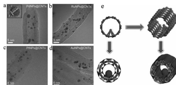
Fig. 5 (a–d) HRTEM images of PdNPs@CNTs (a), RuNPs@CNTs (b), PtNPs@CNTs (c) and AuNPs@CNT (d); (e) schematic illustration of the formation of UMNPs@CNTs (adapted with permission from ref. 59 @ copyright 2014 WILEY-VCH Verlag GmbH & Co. KGaA, Weinheim).
