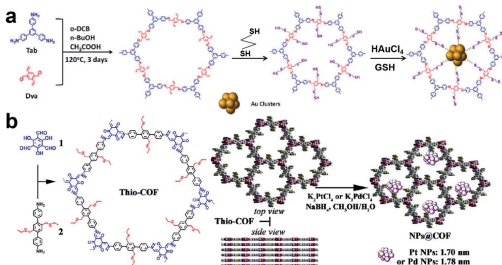
**Fig. 11** (a) Installation of thio groups through the post-synthetic approach: synthesis of Au@COF (o-DCB: 1,2-dichlorobenzene, GSH: glutathione); (b) installation of thio groups through the bottom-up synthetic approach: synthesis of Thio-COF and schematic representation of the synthesis of Thio-COF supported PtNPs@COF and PdNPs@COF (adapted with permission from ref. 25 and 84 @ copyright 2020 Wiley-VCH Verlag GmbH & Co. KGaA, Weinheim and 2017 American Chemical Society).
