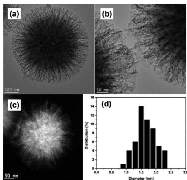
Fig. 16 (a and b) HR-TEM images, (c) HAADF-STEM images and (d) size distribution histogram of KCC-1-NH<sub>2</sub> supported Au UMNPs (adapted with permission from ref. 107 @ copyright 2016 Wiley-VCH Verlag GmbH & Co. KGaA, Weinheim).
