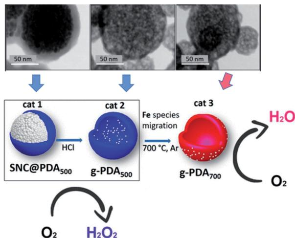
Fig. 6 Under different pyrolysis conditions,  $\text{FeO}_x$  particles were formed on different locations of CNTs as shown in the TEM images. Correspondingly, different ORR product selectivities were observed (SNC: superparamagnetic nanoparticle clusters, PDA: polydopamine) (adapted with permission from ref. 61 @ copyright 2019 American Chemical Society).
