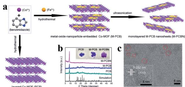
**Fig. 9** (a) Schematic of embedding FeO in the lattice of the MOF; (b) powder XRD patterns of PCB, FeCoO<sub>x</sub> UMNPs-PCB, and FeCoO<sub>x</sub> UMNPs-PCBN; and (c) HRTEM image of FeCoO<sub>x</sub> UMNPs-PCBN (adapted with permission from ref. 77 @ copyright 2020 American Chemical Society).
