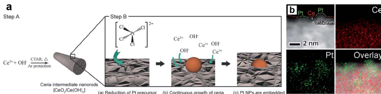
Fig. 13 (a) Schematic illustration of the proposed mechanism of synthesizing surface-embedded Pt/CeO<sub>2</sub> hybrid nanorods and (b) HAADF-STEMEDX mapping images of Pt/CeO<sub>2</sub> hybrid nanorods (adapted with permission from ref. 98 @ copyright 2017 WILEY-VCH Verlag GmbH & Co. KGaA, Weinheim).
