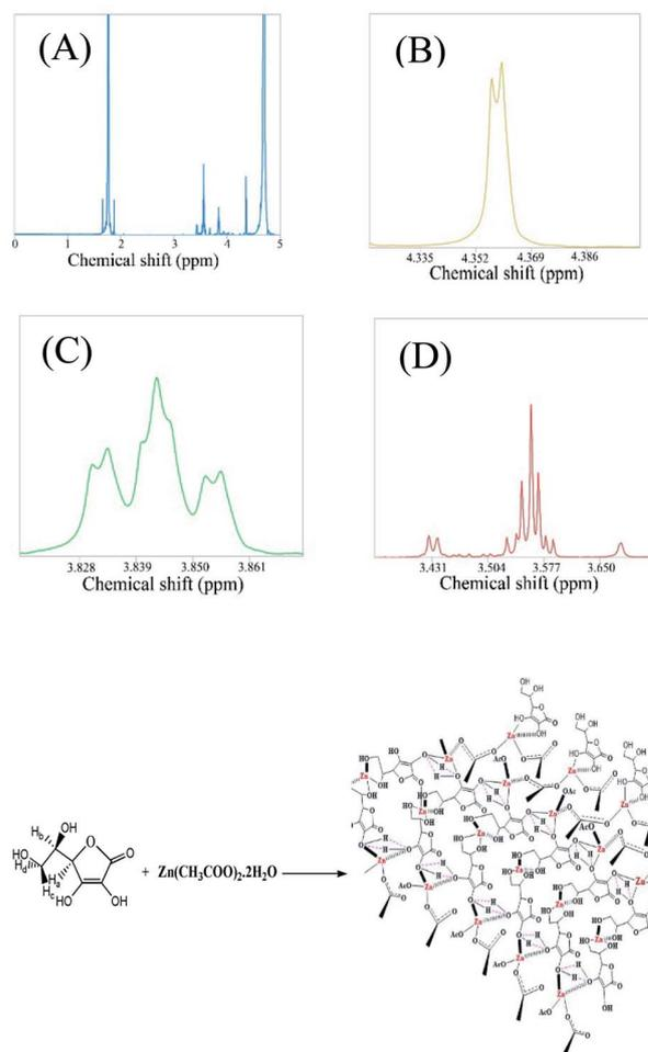
Fig. 9 (A) NMR spectrum of  $Zn_x(AA)_y(OAc)_z$ . (B) Magnified view of the peak shown in (A) at 4.35 for  $H_a$ . (C) Magnified view of the peak shown in (A) at 3.84 for  $H_b$ . (D) Magnified view of the peak shown in (A) at 3.56 for  $H_c$  and  $H_d$ . A schematic representation of the nanoparticle formation from the reaction between ascorbic acid and zinc acetate dihydrate.
