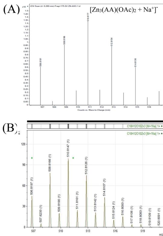
Fig. 8 (A) Experimental mass spectrum of the luminescent dispersion indicating the presence of  $Zn_3(AA)(OAc)_2$ . (B) Simulated mass spectrum of  $Zn_3(AA)(OAc)_2$ .
