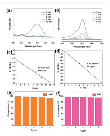
Fig. 5 Time-dependent UV-vis spectral monitoring of the reductive degradation of (a) 4-NP using  $SiO_2$ -g-P4VP/AuNPs as a catalyst at 3 min intervals and (b) RhB using  $SiO_2$ -g-P4VP/AgNPs as a catalyst at 2 min intervals. Plots of  $In(C_t/C_0)$  vs. reaction time for the reductive degradation of (c) 4-NP and (d) RhB. The reusability of (e)  $SiO_2$ -g-P4VP/AuNPs for the reduction of 4-NP and (f)  $SiO_2$ -g-P4VP/AgNPs for the reduction of RhB after five rounds of cycling.
