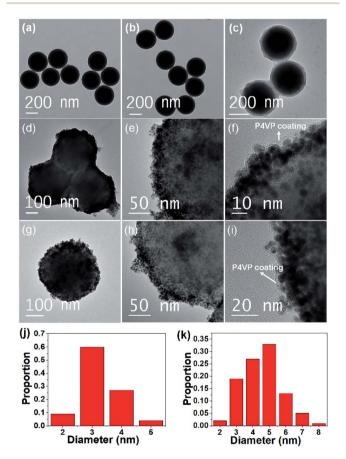
Fig. 3 TEM images of (a) bare silica nanospheres, (b) SiO<sub>2</sub>-Cl, (c) SiO<sub>2</sub>g-P4VP, (d) SiO<sub>2</sub>-g-P4VP/AuNPs and (g) SiO<sub>2</sub>-g-P4VP/AgNPs. HRTEM images of (e and f)  $SiO_2$ -g-P4VP/AuNPs and (h and i)  $SiO_2$ -g-P4VP/ AgNPs. Size distribution histograms of MNPs on (j) SiO<sub>2</sub>-g-P4VP/ AuNPs and (k) SiO<sub>2</sub>-g-P4VP/AgNPs, corresponding to TEM images in (d) and (g), respectively
