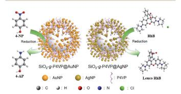
Fig. 6 Schematic illustration of the reductive degradation of 4-NP and RhB using  $SiO_2$ -g-P4VP/MNPs as heterogeneous catalysts.
