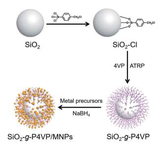
Fig. 1 Schematic illustration of the fabrication of SiO<sub>2</sub>-g-P4VP/MNPs in which MNPs are embedded in the hairy P4VP matrix on the silica core
