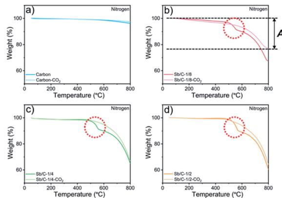
**Fig. 3** TGA profiles of pure carbon and Sb/C nanohybrids tested under a nitrogen atmosphere: carbon and carbon–CO<sub>2</sub> (a), Sb/C-1/8 and Sb/C-1/8-CO<sub>2</sub> (b), Sb/C-1/4 and Sb/C-1/4-CO<sub>2</sub> (c), Sb/C-1/2 and Sb/C-1/2-CO<sub>2</sub> (d). **A** refers to the percentage of mass loss from Sb evaporation under N<sub>2</sub> conditions (50–800 °C).
