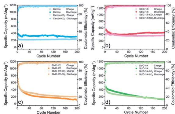
Fig. 4 Cycling performance of pure carbon and Sb/C nanohybrid anodes in LIBs measured at 66 mA g<sup>-1</sup>: carbon and carbon-CO<sub>2</sub> (a), Sb/C-1/8 and Sb/C-1/8-CO<sub>2</sub> (b), Sb/C-1/4 and Sb/C-1/4-CO<sub>2</sub> (c), Sb/C-1/2 and Sb/C-1/2-CO<sub>2</sub> (d).
