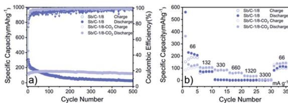
Fig. 7 Cycling (a) and rate (b) performances of Sb/C-1/8 and Sb/C-1/8-CO<sub>2</sub> samples in SIBs. Cycling tests are measured at 66 mA g<sup>-1</sup>, and rate tests are measured from 66 mA g<sup>-1</sup> to 3300 mA g<sup>-1</sup>.
