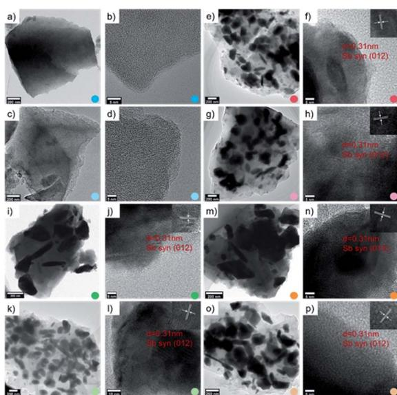
Fig. 1 TEM and HRTEM images of carbon (a, b), carbon-CO<sub>2</sub> (c, d), Sb/C-1/8 (e, f), Sb/C-1/8-CO<sub>2</sub> (g, h), Sb/C-1/4 (i, j), Sb/C-1/4-CO<sub>2</sub> (k, l), Sb/C-1/2 (m, n) and Sb/C-1/2-CO<sub>2</sub> (o, p).
