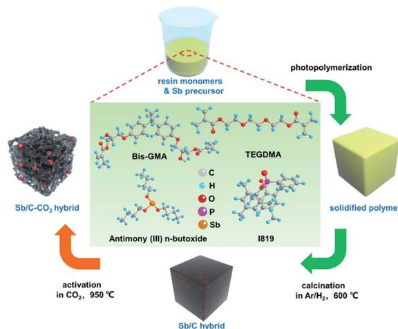
Scheme 1 Schematic illustration of the preparation process of the Sb-based nanohybrids without CO<sub>2</sub> activation (Sb/C hybrid) and with CO<sub>2</sub> activation (Sb/C–CO<sub>2</sub> hybrid).
