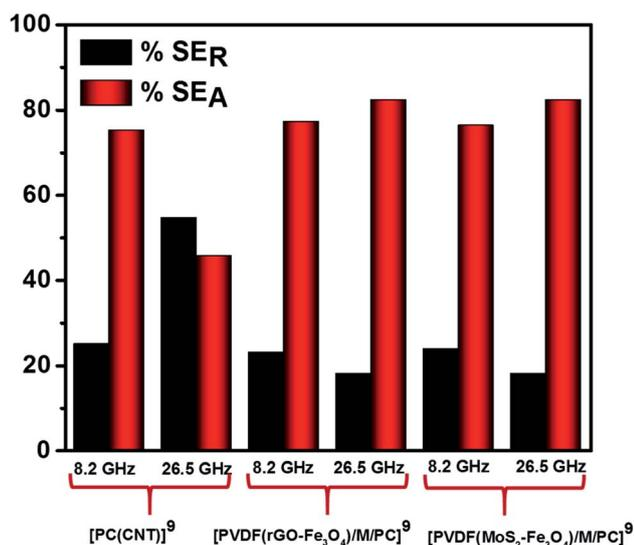
Fig. 12  $SE_A$  and  $SE_R$  for [PC(CNT)]<sup>9</sup>, [PVDF(rGO- $Fe_3O_4$ )/M/PC]<sup>9</sup> and [PVDF(MoS<sub>2</sub>- $Fe_3O_4$ )/M/PC]<sup>9</sup> at 8.2 and 26.5 GHz frequency.
