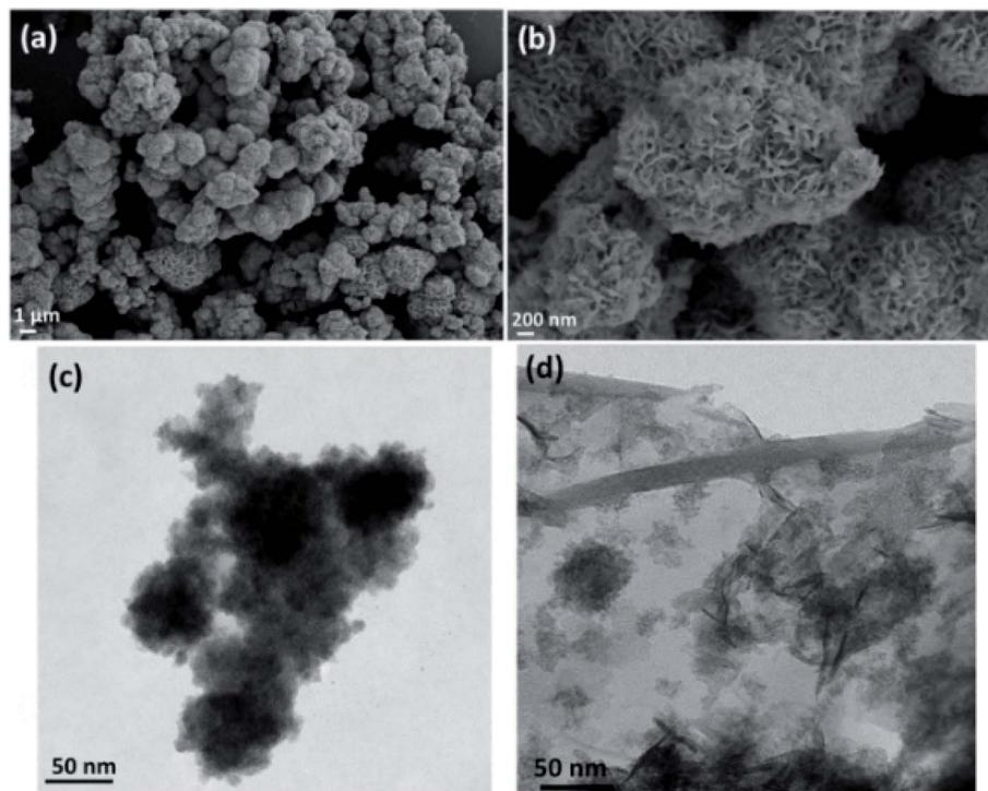
Fig. 2 (a and b) SEM micrograph of MoS<sub>2</sub>, (c) TEM micrographs of MoS<sub>2</sub>-Fe<sub>3</sub>O<sub>4</sub>, and (d) TEM micrograph of rGO-Fe<sub>3</sub>O<sub>4</sub>.
