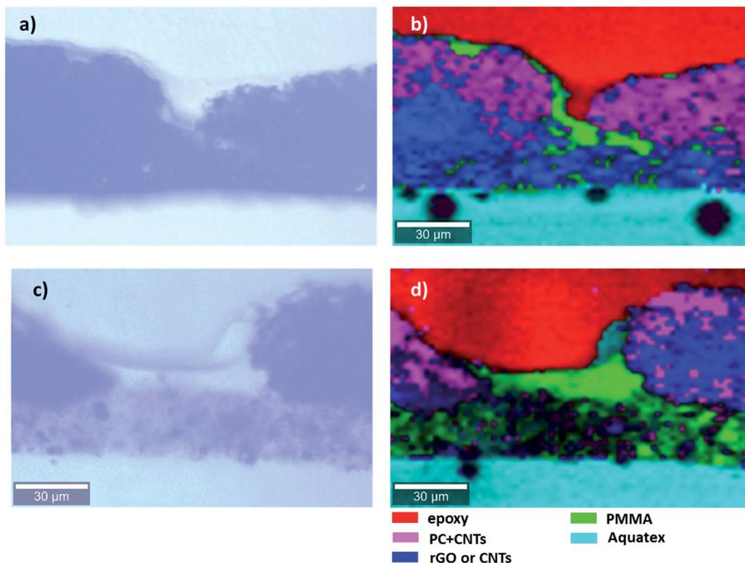
Fig. 7 Light microscopy images (a and c) and Raman map (b and d) of the cross section of the multilayered film: (a and b) PVDF( $rGO-Fe_3O_4$ )/M/PC; (c and d) PVDF( $MoS_2-Fe_3O_4$ )/M/PC.
