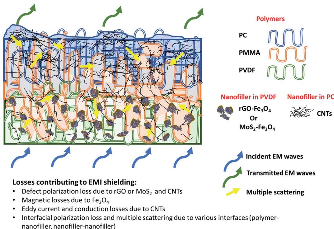
Scheme 4 Loss mechanism involved in the multilayered assembly.
