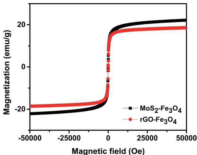
Fig. 4 VSM plot of the synthesized nanoparticles.
