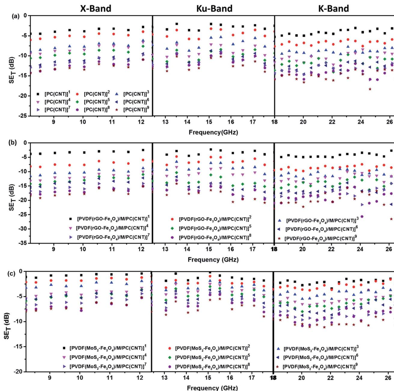
Fig. 11  $SE_T$  vs. frequency for (a) PC(CNT)- set of 9 stacks in an ascending order, (b) PVDF(rGO-Fe<sub>3</sub>O<sub>4</sub>)/M/PC – set of 9 stacks in an ascending order and (c) PVDF(MoS<sub>2</sub>-Fe<sub>3</sub>O<sub>4</sub>)/M/PC – set of 9 stacks in an ascending order. Note that the legend is common for the plots in one row, i.e., for one type of sample across different frequency bands.
