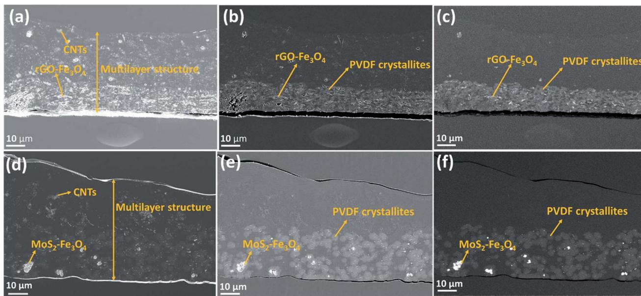
Fig. 5 SEM micrographs of the multilayered film's cross-section (embedded in epoxy and cut using an ultramicrotome). (a–c) PVDF(rGO-Fe<sub>3</sub>O<sub>4</sub>)/M/PC (d–f): PVDF(MoS<sub>2</sub>-Fe<sub>3</sub>O<sub>4</sub>)/M/PC. Each row depicts the same area with different detectors: in-lens, SE2, and back-scattered electrons detectors, respectively.
