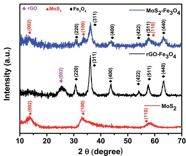
Fig. 1 XRD pattern of MoS<sub>2</sub>, rGO-Fe<sub>3</sub>O<sub>4</sub>, and MoS<sub>2</sub>-Fe<sub>3</sub>O<sub>4</sub>.
