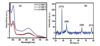
Fig. 4 (a) UV-Vis absorption spectra acquired for DCM solutions of LC-GNPs; notice bands arising due to  $n-\pi^*$  (~300 nm) transition and SPR (~530 nm) pertaining into GNPs. (b) Representative XRD pattern of the as-prepared LC-GNP-4.
