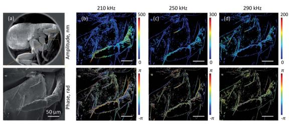
Fig. 3 Hyperspectral imaging of driven oscillations of flea setae. (a) Static secondary electron image of the entire flea and enlarged detail of the motion-imaged area. (b–d) Amplitude (upper row) and corresponding phase (lower) of secondary electron signal modulation at selected driving frequencies [as labelled].
