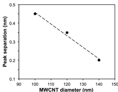
Fig. 5 Plot of peak separation in the oscillations observed for the electrical resistance of an individual MWCNT (determined from 3PP  $I$ - $V$  measurements caused by distortion induced by pressure applied by a central "floating" probe) as a function of the MWCNT diameter.
