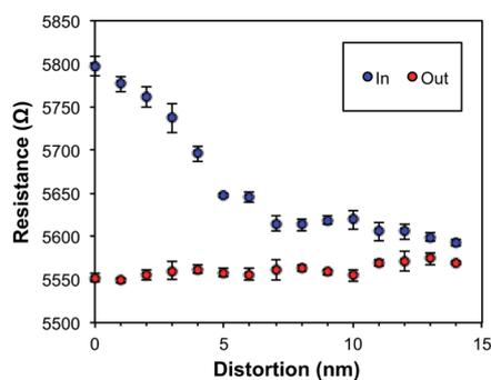
Fig. 2 Plot of the electrical resistance of an individual MWCNT as determined from 2PP  $I$ - $V$  measurements as a function of distortion induced by pressure applied by one of the probes (measured as the extension of the piezo that controls the tip). The blue circle data points show the values with the depression of the probe and the red circle data points show the resistance upon relaxation of distortion by removal of the probe (error bars show the standard error).
