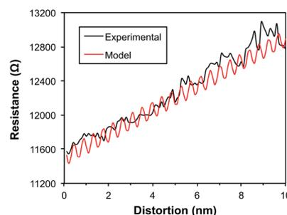
Fig. 3 Plot of the electrical resistance of an individual MWCNT as determined from 3PP  $I$ - $V$  measurements as a function of distortion, induced by pressure applied by the central "floating" probe, distortion (measured as the extension of the piezo that controls the tip) (black line) and calculated fit (red line) highlighting the oscillations.
