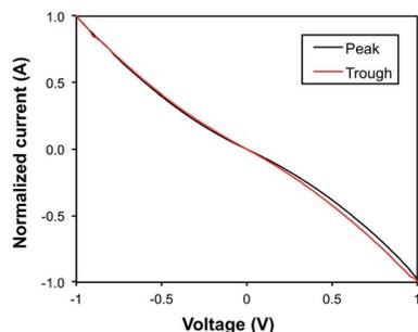
Fig. 4 Normalised  $I$ - $V$  curves of a typical resistance peak (black line) and adjacent resistance trough (red line) in the oscillations observed for the electrical resistance of an individual MWCNT determined from 3PP  $I$ - $V$  measurements caused by distortion induced by pressure applied by a central "floating" probe, shown in Fig. 3.
