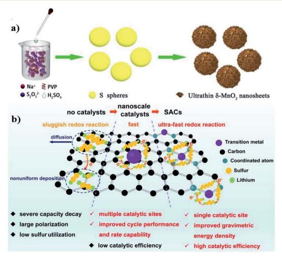
Fig. 9 (a) Schematic illustration for the synthesis of sulfur nanospheres and sulfur nanospheres@ultrathin  $\delta$ -MnO<sub>2</sub> nanosheet core-shell structures, and the conversion of Li<sub>2</sub>S<sub>x</sub> on the core-shell surface. <sup>101</sup> Reproduced with permission. Copyright 2020 American Chemical Society. (b) Catalytic mechanism of SACs for sulfur electrodes. <sup>102</sup> Reproduced with permission. Copyright 2021 Elsevier.
