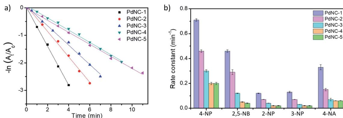
Fig. 4 (a) Comparative rate constant plot of  $-\ln(A_t/A_0)$  vs. time for 4-NP reduction using the different PdNCs, (b) comparison of the rate-constants exhibited by the different PdNCs for the reduction of 4-NP, 2,5-NB, 2-NP, 3-NP and 4-NA.
