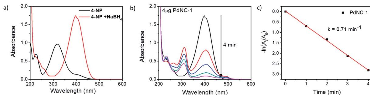
Fig. 3 (a) UV-vis absorption spectra of 4-NP before and after the addition of  $NaBH_4$ , (b) time-dependent UV-vis absorption spectra of the 4-NP in presence of  $NaBH_4$  and 4  $\mu$ g of PdNC-1 and (c) the corresponding rate-constant plot of  $-\ln(A_t/A_0)$  vs. time.
