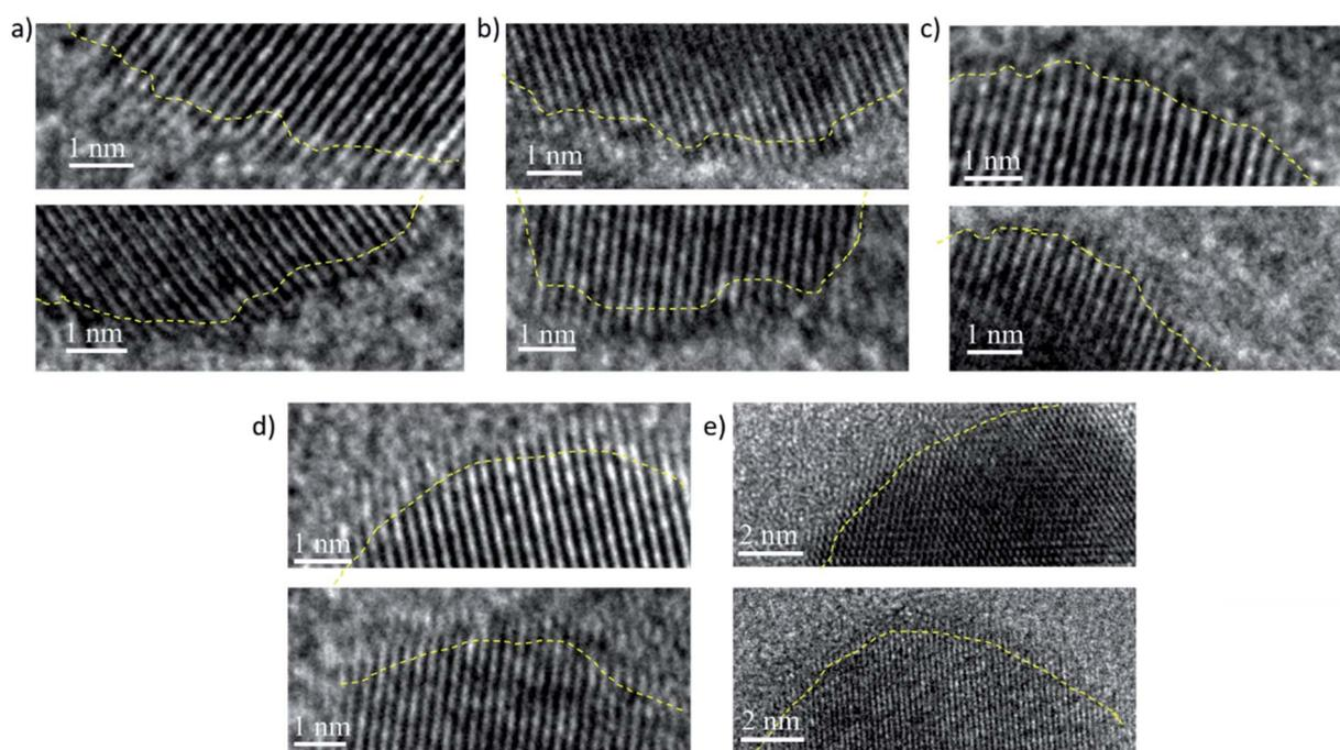
Fig. 6 Typical high-resolution TEM images recorded at the nanocrystal edges showing the presence of defects and the different extent of deviations from an ideal spherical shape for (a) PdNC-1, (b) PdNC-2, (c) PdNC-3, (d) PdNC-4 and (e) PdNC-5. The yellow lines a guide to the eye.
