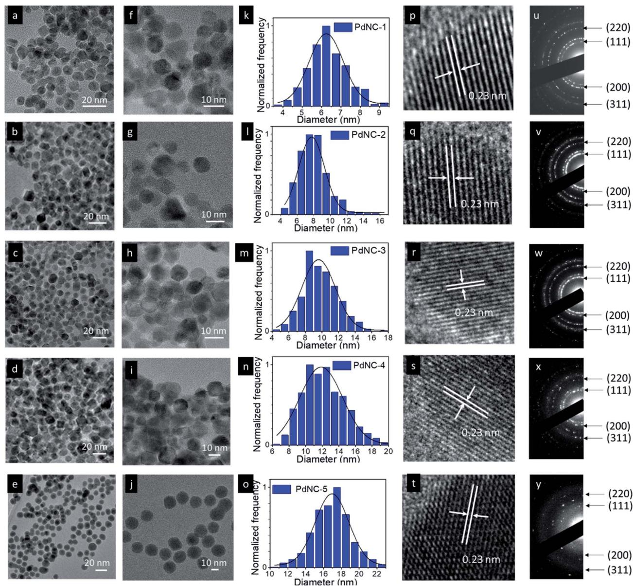
Fig. 1 Low magnification TEM images of (a and f) PdNC-1, (b and g) PdNC-2, (c and h) PdNC-3, (d and i) PdNC-4, (e and j) PdNC-5. Particle size distribution histogram of (k) PdNC-1, (l) PdNC-2, (m) PdNC-3, (n) PdNC-4, (o) PdNC-5. HRTEM images of (p) PdNC-1, (q) PdNC-2, (r) PdNC-3, (s) PdNC-4, (t) PdNC-5 and indexed SAED patterns of (u) PdNC-1, (v) PdNC-2, (w) PdNC-3, (x) PdNC-4, (y) PdNC-5.
