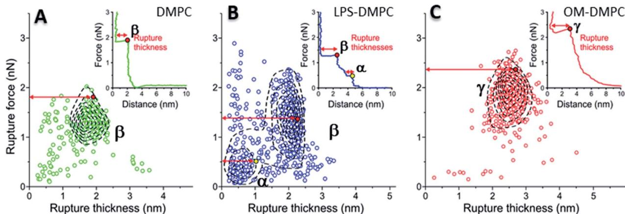
Fig. 8 2D maps of the distribution of rupture events of solid-phase DMPC (A), LPS-DMPC (B), OM-DMPC (C) ( $n = 400$  for all data sets, but not every point is shown for clarity). Insets show a typical force–distance curve recorded while piercing through the corresponding samples. Red and yellow colored dots explain the difference between “Distance” and “Rupture distance”. Greek letters show populations of breakthrough events. FS measurements were always done at 20 °C.
