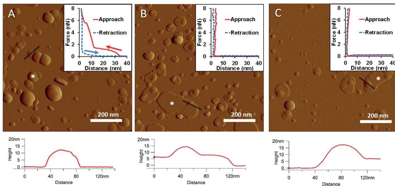
Fig. 2 Amplitude-contrast AFM image of LPS vesicles in the presence of 10 mM  $\text{Ca}^{2+}$ ; at 20 °C (A). The sample was warmed to 50 °C (B); and then cooled back to 20 °C (C). Insets: force–distance curves recorded while pressing LPS at the locations marked by the white star on each image. On the inset of A arrows indicate the direction of tip movement. Lower panels show height profiles taken along the black lines.
