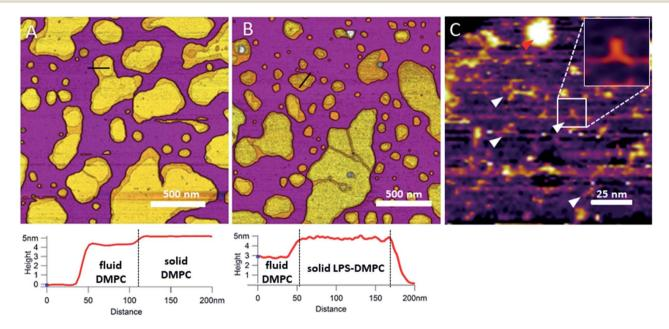
Fig. 3 Height-contrast AFM image of DMPC SLB (A); LPS-DMPC SLB (B); and an LPS-rich region of LPS-DMPC SLB at high resolution (C); on mica at 20 °C in the presence of 10 mM Ca<sup>2+</sup>. Lower panels show the height-distance functions along the black lines shown in the images. In C the putative branching LPS oligosaccharide chains are marked with white arrowheads; one of them is enlarged in the top right inset. Red arrowhead indicates an LPS bump.
