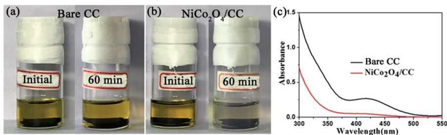
Fig. 6 Polysulfide adsorption properties of CC and NiCo<sub>2</sub>O<sub>4</sub>/CC. Visual experiments with (a) CC and (b) NiCo<sub>2</sub>O<sub>4</sub>/CC placed in the solution of Li<sub>2</sub>S<sub>4</sub>/DOL/DME (2 mmol, DOL : DME volume ratio 1 : 1) at the beginning and after 60 min. (c) UV-vis absorption curves of Li<sub>2</sub>S<sub>4</sub>/DOL/DME solution after 1 h adsorption by bare CC and NiCo<sub>2</sub>O<sub>4</sub>/CC.
