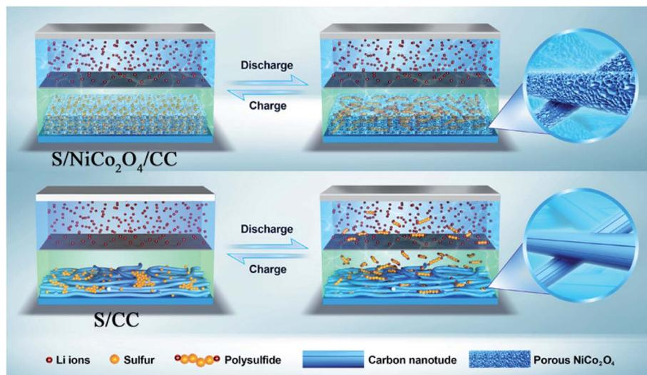
Fig. 8 Schematic illustration of the charge/discharge properties of the Li-S cells with S/NiCo<sub>2</sub>O<sub>4</sub>/CC and S/CC cathodes.
