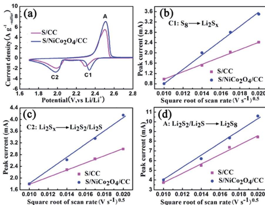
Fig. 7 (a) CV curves for S/CC and S/NiCo<sub>2</sub>O<sub>4</sub>/CC at 0.4 mV s<sup>-1</sup>. (b–d) Plots of the peak current against the square root of scan rate for peaks C1, C2 and A.
