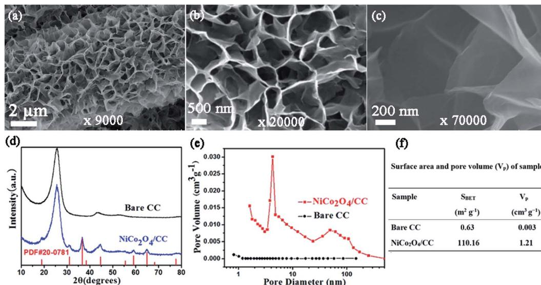
Fig. 2 Characterization of NiCo<sub>2</sub>O<sub>4</sub>/CC. SEM images of the NiCo<sub>2</sub>O<sub>4</sub> nanosheets with magnifications of (a) 9000, (b) 20 000 and (c) 70 000, respectively. (d) XRD patterns of NiCo<sub>2</sub>O<sub>4</sub>/CC and CC. (e) Pore size distribution of NiCo<sub>2</sub>O<sub>4</sub>/CC and CC. (f) Surface area and pore volume of NiCo<sub>2</sub>O<sub>4</sub>/CC and CC.
