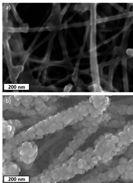
Fig. 5 SEM images of (a) pristine CNT ribbons and (b) decorated CNT/Cu-NPs.
