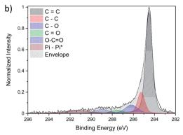
Fig. 7 Comparison of the high-resolution C 1s XPS spectra of (a) pristine CNTs and (b) CNT/Cu-NP composite.
