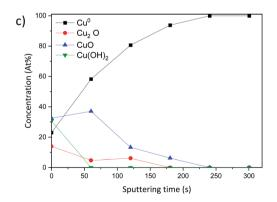
Fig. 4 Curve fitting of the high resolution spectra of copper Cu 2p obtained by X-ray photoelectron spectroscopy using depth profile during 300 s; (a) as-deposited sample without sputtering, (b) sample with 30 s Ar<sup>+</sup> sputtering and (c) evolution of the concentration of the different peaks fitted as a function of the sputtering time of Cu-NPs deposited on a Si substrate
