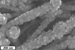
Fig. 5 SEM images of (a) pristine CNT ribbons and (b) decorated CNT/ Cu-NPs.
