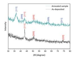
Fig. 3 X-ray diffraction spectrum of the as-deposited Cu-NPs (black) and annealed for 20 min at 120 °C (dark cyan) deposited on a silicon substrate. [Numbers] corresponding plane for Cu (red) and Cu<sub>2</sub>O (blue).
