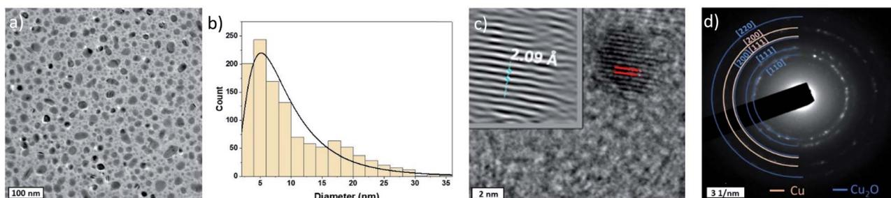
Fig. 2 (a) Low resolution TEM image of the as deposited Cu-NPs; (b) size distribution of TEM images; (c) high resolution TEM image and *d*-spacing of the [111] and [200] planes of Cu and (d) selected area electron diffraction (SAED) pattern of the sample.
