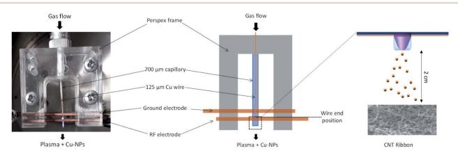
Fig. 1 Photograph of the real plasma reactor and the corresponding schematic drawn.
