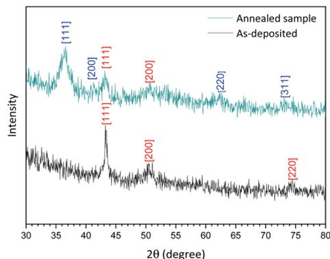
Fig. 3 X-ray diffraction spectrum of the as-deposited Cu-NPs (black) and annealed for 20 min at 120 °C (dark cyan) deposited on a silicon substrate. [Numbers] corresponding plane for Cu (red) and  $\text{Cu}_2\text{O}$  (blue).
