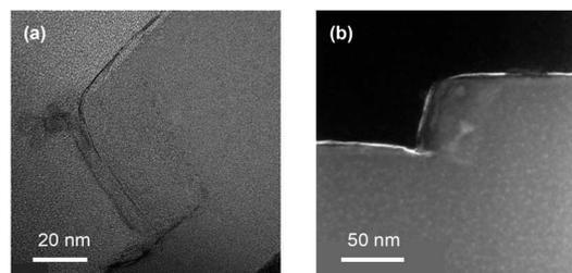
Fig. 2 (a) High-resolution and (b) high angle annular dark-field scanning transmission electron microscopy images of the conformally grown MoS<sub>2</sub> layers on the NP-patterned SiO<sub>2</sub>/Si substrates.
