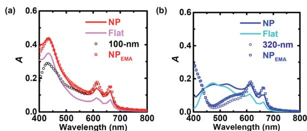
Fig. 5 FDTD calculated optical absorption in the  $\text{MoS}_2$  monolayers ( $A$ ) on the NP and flat regions formed in (a) 100 and (b) 320 nm- $\text{SiO}_2/\text{Si}$  wafers. For comparison,  $A$  of non-patterned 100 and 320 nm- $\text{SiO}_2/\text{Si}$  wafers are also included: 100 nm in (a) and 320 nm in (b).  $A$  on the NP regions was also estimated using the EMA method, as indicated as  $\text{NP}_{\text{EMA}}$  in (a) and (b).
