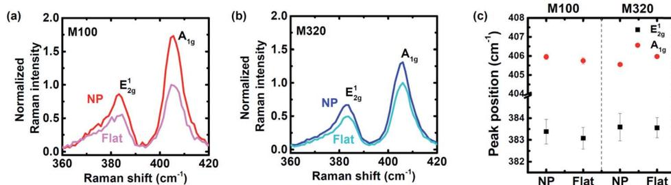
Fig. 4 Raman spectra of (a) M100 and (b) M320. The intensity was normalized with respect to the  $A_{1g}$  peak intensity of the flat region for each sample. (c)  $E_{2g}^1$  and  $A_{1g}$  peak positions of the NP and flat regions for M100 and M320. The spectra from the NP and flat regions are obtained from each sample using micron-sized laser beams.
