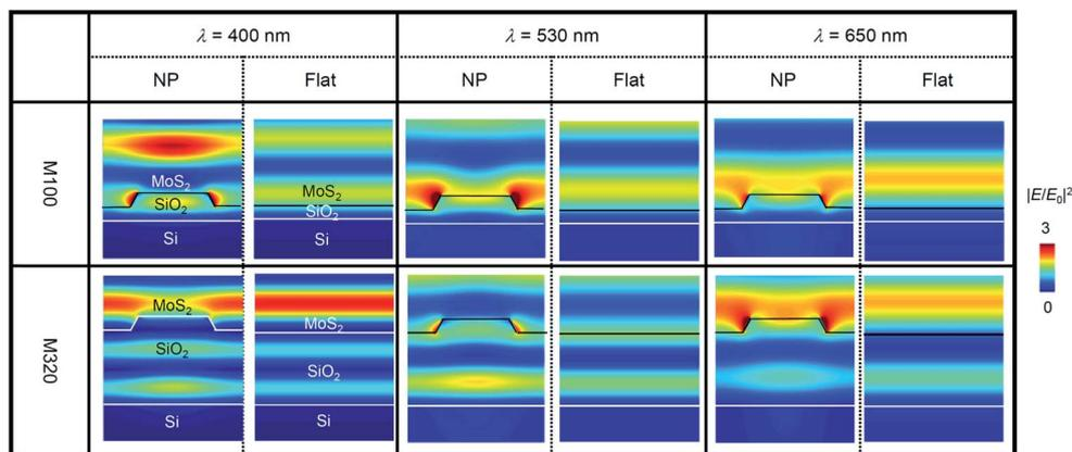
Fig. 6 Cross-sectional distributions of the E-field intensity ( $|E/E_0|^2$ , where  $E_0$  represents the magnitude of the E-field of the incident light) in the MoS<sub>2</sub>-monolayer-coated NP and flat regions for M100 and M320 at  $\lambda = 400, 530, \text{ and } 650 \text{ nm}$ .
