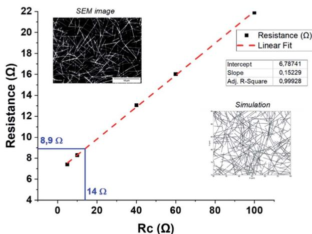
Fig. 2 Determination of the average contact resistance between AgNWs: the simulated network sheet resistance is plotted *versus* the contact resistance ( $R_c$ ) between two AgNWs. The computed  $R_s$  value is finally adjusted to the experimental one, leading to the correct estimated  $R_c$  value. SEM pictures of AgNW networks are used to extract the network density. For each arbitrary  $R_c$  value, 50 simulations were performed in order to average the randomness of the simulated networks.
