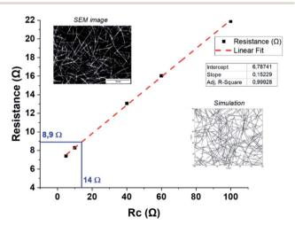
Fig. 2 Determination of the average contact resistance between AgNWs: the simulated network sheet resistance is plotted versus the contact resistance ( $R_c$ ) between two AgNWs. The computed  $R_s$  value is finally adjusted to the experimental one, leading to the correct estimated  $R_c$  value. SEM pictures of AgNW networks are used to extract the network density. For each arbitrary  $R_c$  value, 50 simulations were performed in order to average the randomness of the simulated networks.
