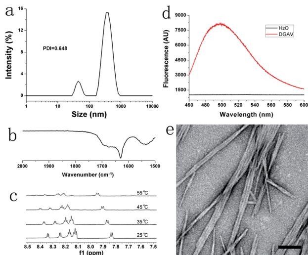
**Fig. 2** Formation of nanofibers from DGAV in pH 2.0 solution. (a) DLS revealing size distribution between 10 and 1000 nm. (b) FTIR spectrum and (c) temperature-dependent NMR spectra indicating the formation of intermolecular hydrogen bonds. (d) ThT-binding fluorescence indicating the formation of amyloid-like aggregates. (e) TEM showing the formation of self-aggregating nanofibers. Scale bar = 100 nm.
