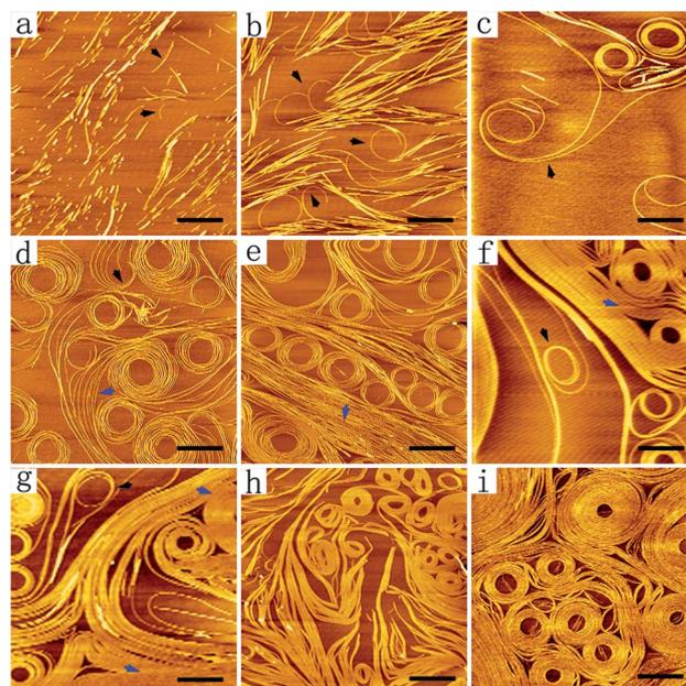
**Fig. 3** AFM images of patterns formed by DGAV nanofibers after being incubated on a mica surface for (a) 0 min, (b) 5 min, (c) 30 min, (d) 1 h, (e) 1.5 h, (f) 2 h, (g) 6 h, (h) 12 h and (i) 24 h. Scale bars = 1  $\mu\text{m}$ .
