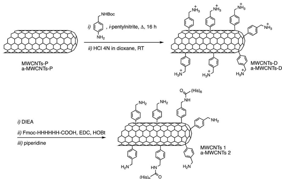
Fig. 1 Synthesis of derivatives MWCNTs 1 and a-MWCNTs 2.
