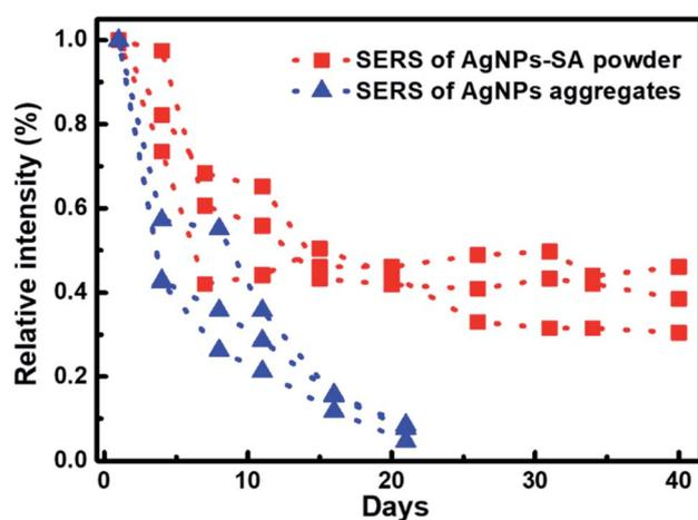
Fig. 4 SERS stability of the AgNPs-SA powder. Squares and triangles demonstrate the SERS intensity ( $I_{1436\text{ cm}^{-1}}$  of 4-ATP) evolutions of 3D AgNPs-SA powder and conventional 2D AgNPs aggregates with different preserved time in ambient condition, respectively. For comparison, three groups of controlled experiments were done. The dash lines are plotted to guide eyes.
