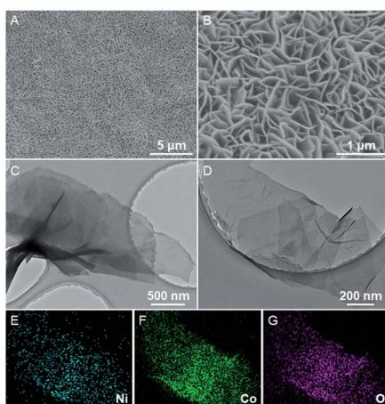
Fig. 2 SEM (A and B) and TEM (C and D) images of Ni–Co(OH)<sub>2</sub> NSAs. Mapping images of different elements for the nanosheets of Ni (E), Co (F) and O (G).
