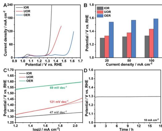
Fig. 3 (A) Polarization curves of the IOR, UOR and OER over Ni-Co(OH)<sub>2</sub> NSAs. (B) Comparison of potentials required to drive different current densities of the IOR, UOR and OER over Ni-Co(OH)<sub>2</sub> NSAs. (C) Tafel plots of electrooxidation reactions from (A). (D) Chronopotentiometry curve of the IOR over Ni-Co(OH)<sub>2</sub> NSAs.
