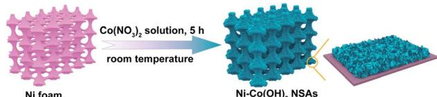
Fig. 1 Schematic illustration of the fabrication of Ni–Co(OH)<sub>2</sub> NSAs.
