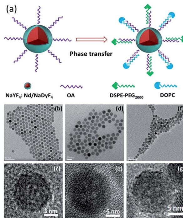
Fig. 1 (a) Schematic illustration of Lipo- $\text{NaYF}_4:\text{Nd}/\text{NaDyF}_4$  NCs. Typical and high resolution TEM images of OA- $\text{NaYF}_4:\text{Nd}$  (b and c), OA- $\text{NaYF}_4:\text{Nd}/\text{NaDyF}_4$  (d and e) and Lipo- $\text{NaYF}_4:\text{Nd}/\text{NaDyF}_4$  (f and g) NCs, respectively.
