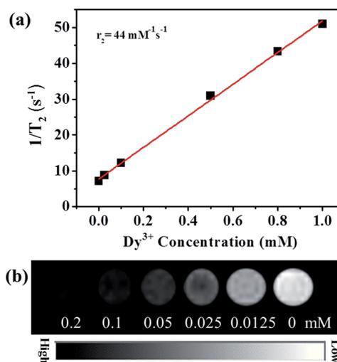
Fig. 5 (a) T<sub>2</sub> relaxivity plot of Lipo-NaYF<sub>4</sub>:Nd/NaDyF<sub>4</sub> NCs dispersed in saline. (b) T<sub>2</sub>-weighted MRI of HeLa cells after being transfected with Lipo-NaYF<sub>4</sub>:Nd/NaDyF<sub>4</sub> NCs using an 11.7 T MR system.
