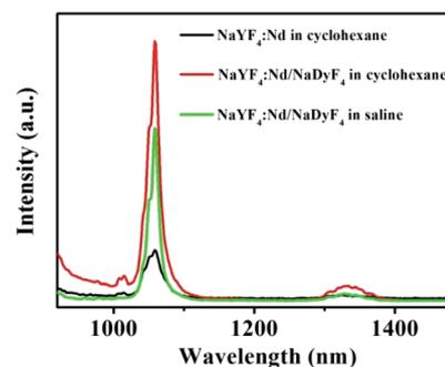
Fig. 3 Luminescence emission spectra of OA- $\text{NaYF}_4\text{:Nd}$  NCs in cyclohexane (black), OA- $\text{NaYF}_4\text{:Nd/NaDyF}_4$  NCs in cyclohexane (red) and Lipo- $\text{NaYF}_4\text{:Nd/NaDyF}_4$  NCs in saline (green) solution under excitation of 785 nm.
