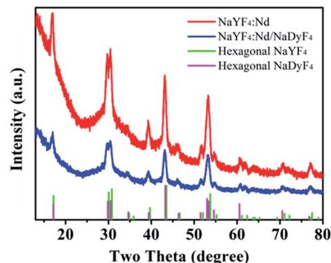
Fig. 2 XRD patterns of the as-synthesized  $\text{NaYF}_4\text{:Nd}$  (red) and  $\text{NaYF}_4\text{:Nd/NaDyF}_4$  (blue) nanoparticles and corresponding standard curves (green, magenta).
