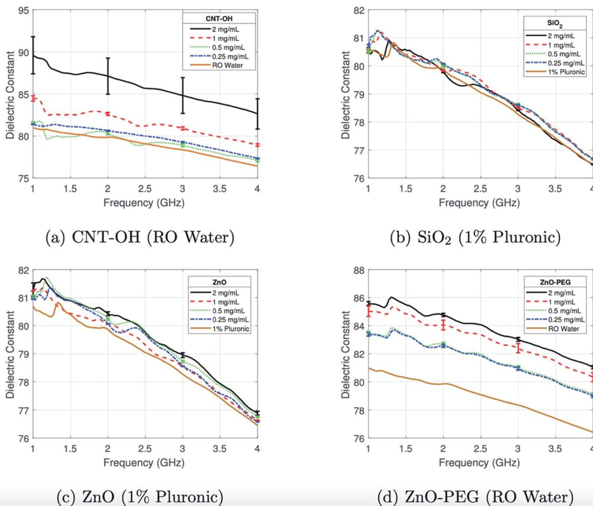
Fig. 3 Average dielectric constant of colloidal dispersions of (a) CNT-OH in RO water, (b) SiO<sub>2</sub> with 1% Pluronic, (c) ZnO with 1% Pluronic, and (d) ZnO-PEG in RO water characterised between 1 and 4 GHz. This figure has been reproduced from ref. 42 with permission from American Association of Physicists in Medicine, copyright 2018.
