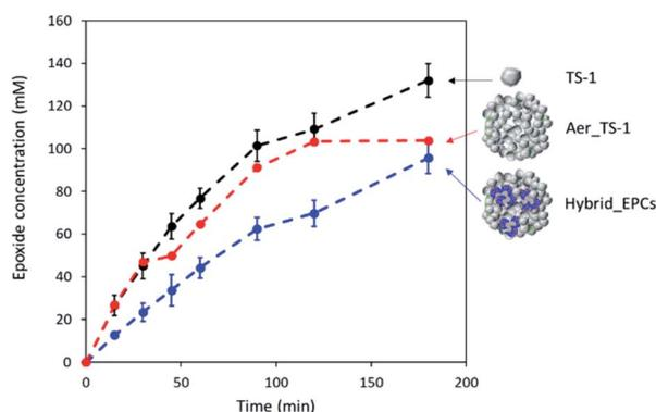
Fig. 3 Kinetic data for the Ti-catalysed conversion of allyl alcohol into glycidol in  $H_2O$  using aqueous solution of hydrogen peroxide as oxidant. Experimental conditions:  $T = 45 \text{ }^\circ\text{C}$ , [catalyst] =  $5 \text{ g L}^{-1}$ ,  $[H_2O_2] = 0.18 \text{ M}$ , [allyl alcohol] =  $0.9 \text{ M}$ . The experiment has been repeated three times with TS-1 and two times with Hybrid\_EPCs to evaluate the experimental error on these measurements (see error bars).
