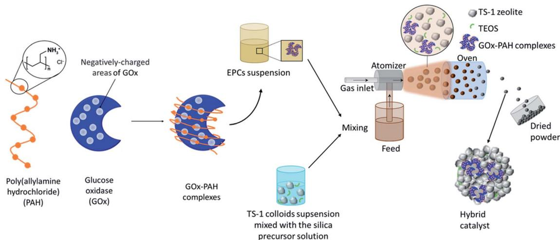
**Scheme 1** Schematic representation of the one-pot synthesis strategy. The EPCs are primarily self-assembled by mixing the PAH and GOx. The TS-1 colloids suspension and the silica precursors solution, mixed beforehand, are mixed with the EPCs suspension.
