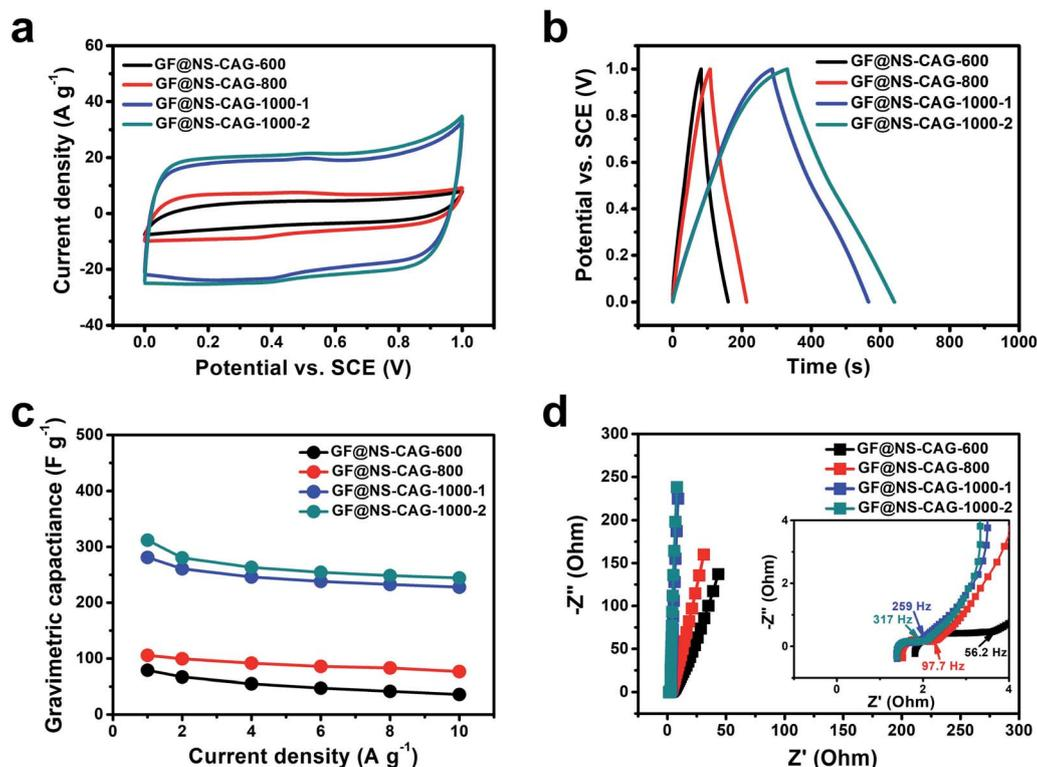
Fig. 5 Electrochemical performances of the GF@NS-CAG electrodes. (a) CV curves at 20 mV s<sup>-1</sup>. (b) GCD curves at 1 A g<sup>-1</sup>. (c) Gravimetric capacitance. (d) Nyquist plots (inset: magnification of the high-frequency region).
