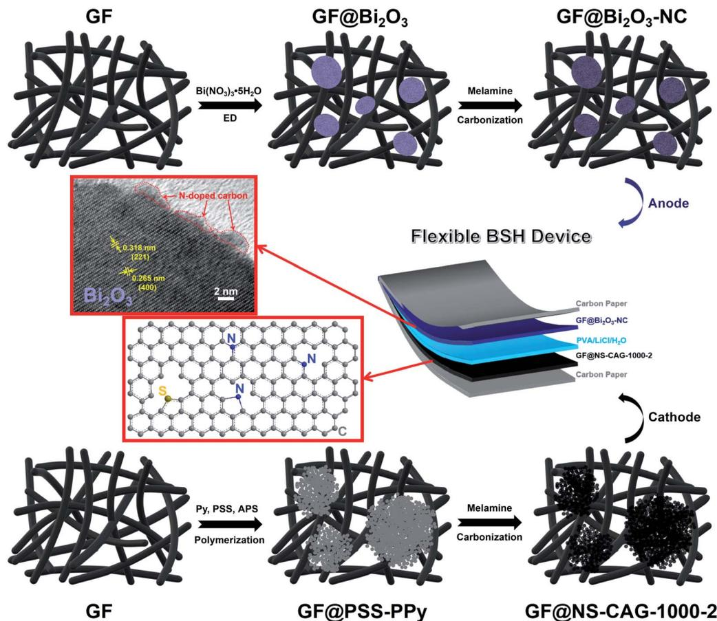
Fig. 1 Schematic illustration of the assembly of a flexible BSH device based on the GF@Bi<sub>2</sub>O<sub>3</sub>-NC anode and the GF@NS-CAG-1000-2 cathode.
