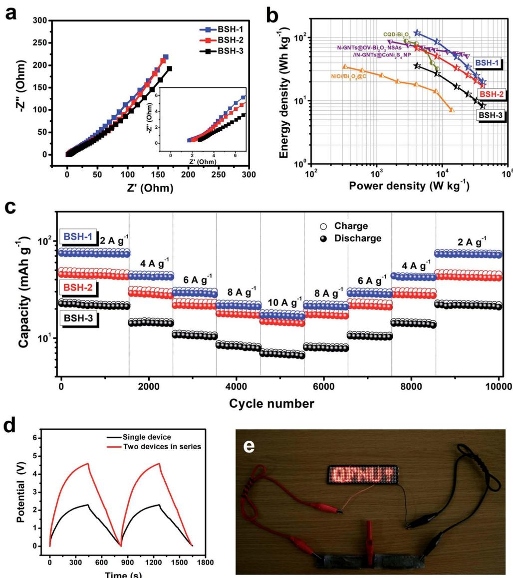
Fig. 7 (a) Nyquist plots (inset: magnification of the high-frequency region). (b) Ragone plots of our devices compared with previously-reported symmetric and asymmetric devices based on  $\text{Bi}_2\text{O}_3$ . (c) Cycling stability obtained by consecutive GCD tests at different current densities for 10 000 cycles in total. (d) GCD curves of two BSH-1 devices connected in series at  $1 \text{ A g}^{-1}$ . (e) A photograph of a red LED array powered by two BSH-1 devices connected in series.
