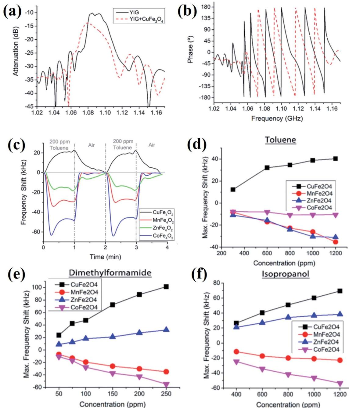
Fig. 13 (a and b) Frequency response of the MSSW-based magnetic gas sensor device before and after being coated with CuFe<sub>2</sub>O<sub>4</sub> nanoparticles. (c) Response of the magnetic gas sensors based on spinel oxides for 200 ppm toluene at room temperature. The response of the magnetic sensors at different concentrations of (d) toluene, (e) dimethylformamide, and (f) isopropanol. Reprinted with permission from ref. 84. Copyright (2017) Elsevier.
