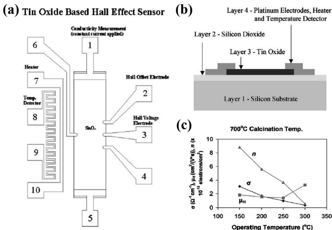
Fig. 4 (a) Tin-oxide based Hall effect sensor. (b) Cross-sectional view of the tin-oxide based Hall effect sensor. (c) Tin oxide thin film conductivity ( $\sigma$ ), electron density ( $n$ ), and Hall mobility ( $\mu_H$ ) in air vs. operating temperature for sensor calcined at 700 °C. Reprinted with permission from ref. 44. Copyright (2001) Elsevier.
