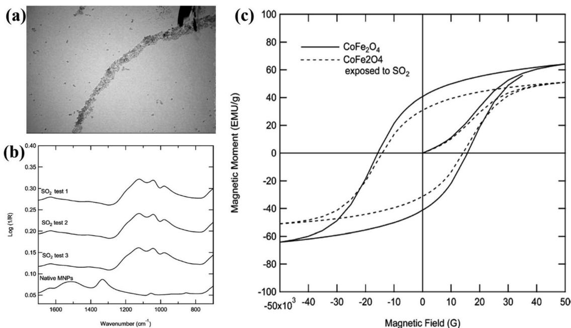
Fig. 3 (a) TEM images of CoFe<sub>2</sub>O<sub>4</sub> MNPs. (b) FTIR spectra of the native MNPs before exposure to sulfur dioxide as well as MNPs after exposure (test 1) and MNPs after exposure but without desorption (tests 2 and 3). (c) Magnetic susceptibility curves for MNPs both before and after sulfur dioxide breakthrough experiments. Reprinted with permission from ref. 33. Copyright (2012) American Chemical Society.
