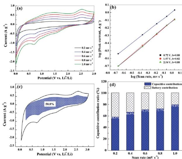
Fig. 7 (a) CV curves of the S-NPC-40 anode at different scan rates, (b)  $b$  value according to the relationship between the peak current and the scan rate, (c) CV curve of the S-NPC-40 anode with the shadowed area representing the surface capacitive contribution, and (d) the proportions of capacitive contribution and battery contribution at different scan rates.
