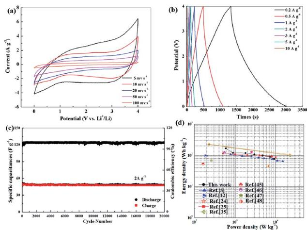
Fig. 9 (a) CV curves of the S-NPC-40//S-NPC-40 LIC within the voltage of  $0$ – $4.0 \text{ V}$  at different scan rates, (b) galvanostatic charge–discharge curves at different current densities, (c) cycling stability of S-NPC-40//S-NPC-40 LIC at a current density of  $2 \text{ A g}^{-1}$ , and (d) Ragone plots of the S-NPC-40//S-NPC-40 LIC compared with previously reported LICs.
