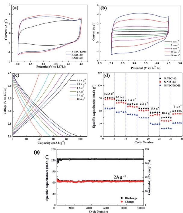
Fig. 8 (a) CV curves of S-NPC-40, S-NPC-60 and S-NPC-KOH cathodes at a scan rate of  $5 \text{ mV s}^{-1}$ , (b) CV curves of the S-NPC-40 cathode at different scan rates, (c) charge–discharge curves of the S-NPC-40 cathode at different current densities, (d) rate performance of S-NPC-40, S-NPC-60 and S-NPC-KOH cathodes, and (e) cycle performance of the S-NPC-40 cathode at a current density of  $2 \text{ A g}^{-1}$  for 2000 cycles.
