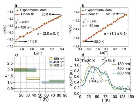
Fig. 5 (a) and (b) Linearization process for the 180 nm nanowire. (c) Power laws extracted from the data linearization (error bar represented by the height). (d) Resistivity derivative.
