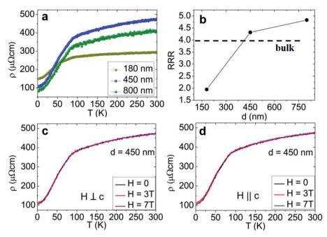
Fig. 4 Single nanowire electrical transport performance. (a) Temperature-dependent resistivity for nanowires of d = 180, 450, 800 nm. (b) Residual resistivity ratio evolution with diameter. Temperature-dependent resistivity with applied magnetic field either perpendicular (c) or parallel (d) to the c-axis (d = 450 nm).
