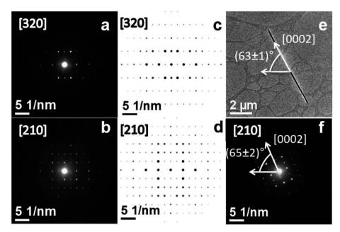
Fig. 3 Mn-Si core microstructural SAED analysis (same nanowire than presented in Fig. 2). (a) and (b) Experimental and (c) and (d) simulated SAED patterns for  $Mn_5Si_3$  crystalline structure. Angle of the nanowire longitudinal direction in the bright-field TEM image (e) and of the [0002] direction in the respective SAED pattern (f).
