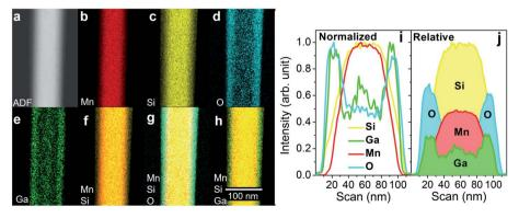
Fig. 2 Nanowire core-shell chemical composition. ADF image (a), and EDS maps indicating the presence of Mn-K $\alpha_{1,2}$ , -L $\alpha_{1}$ , Si K $\alpha_{1,2}$ , -K $\beta_{1}$ , O  $-K\alpha_{1,2}$  and  $Ga-K\alpha_{1,2}$ ,  $-K\beta_1$ ,  $-L\alpha_1$  (b)-(e), respectively, with their color mixtures (f)-(h). (i) and (j) Normalized and relative horizontal element intensity scans, obtained from EDS map integration.
