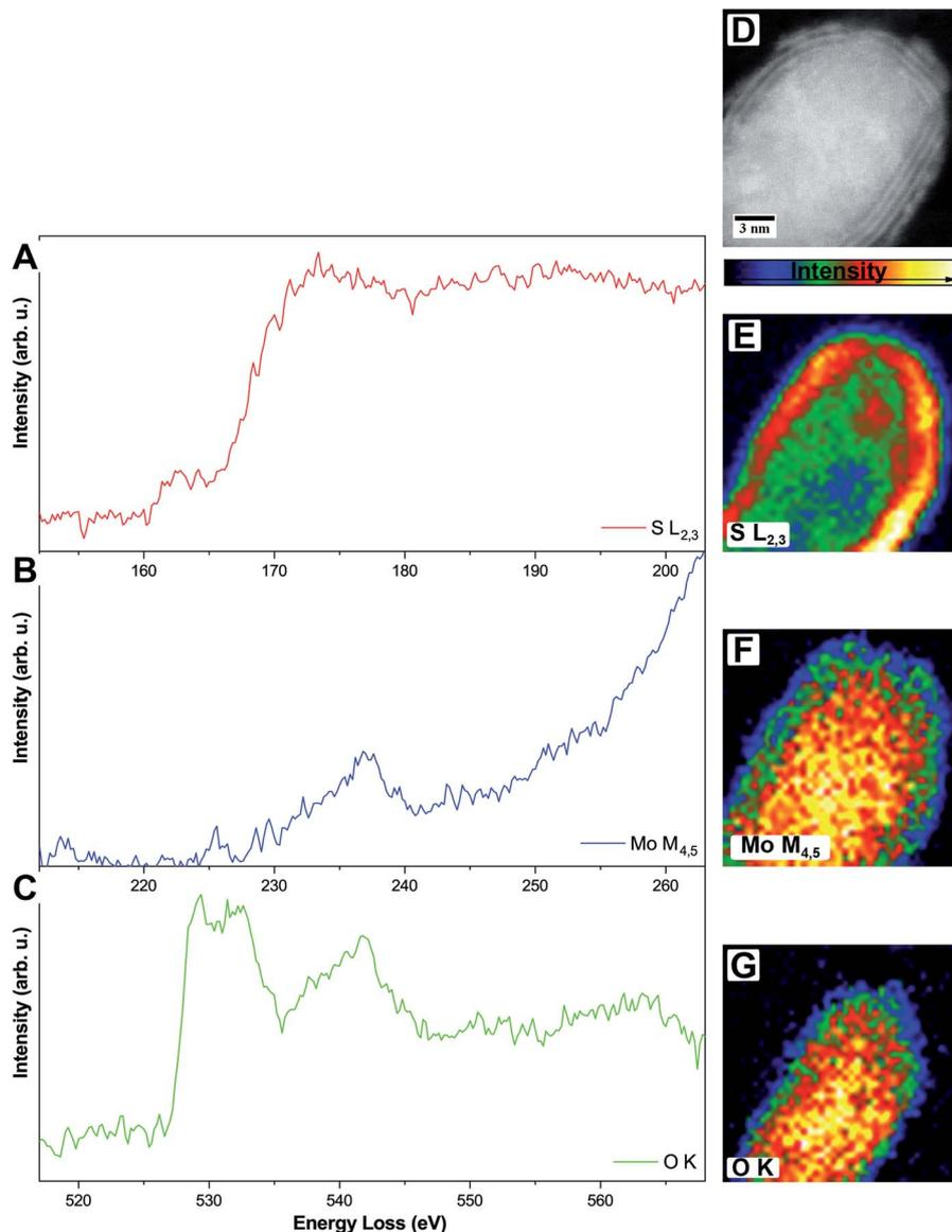
Fig. 4 (A–C) Single-elemental EEL spectra of one MoO<sub>2</sub>/MoS<sub>2</sub> core/shell particle, S-L<sub>2,3</sub> (A), Mo-M<sub>4,5</sub> (B), and O-K (C), respectively. (D–G) HAADF STEM image (D) and intensity-colored single-elemental EELS maps for S-L<sub>2,3</sub> (E), Mo-M<sub>4,5</sub> (F), and O-K (G), respectively.
