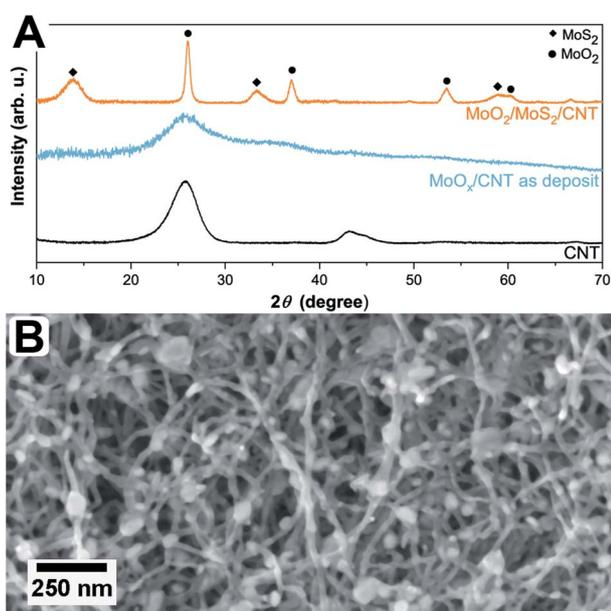
Fig. 1 (A) XRD pattern of uncoated CNTs (bottom, black), as-deposited  $\text{MoO}_x$  on CNTs (middle, blue), and sulfurized  $\text{MoO}_2/\text{MoS}_2$  on CNTs (top, orange). Peaks originating from  $\text{MoS}_2$  and  $\text{MoO}_2$  are marked with  $\blacklozenge$  and  $\bullet$ , accordingly. (B) SEM top view image of  $\text{MoO}_2/\text{MoS}_2$  core/shell nanoparticles within an entangled CNT network.
