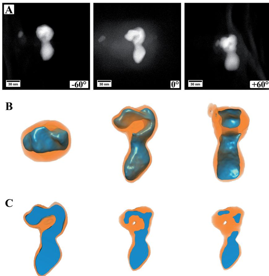
**Fig. 5** Images and reconstructed volume of a  $\text{MoO}_2/\text{MoS}_2$  core/shell particle from the TEM sample prepared on a grid coated with continuous carbon. (A) HAADF STEM images from the tilt series of one area used for reconstruction. Three different angles are shown. (B) The reconstructed volume of the core/shell particle displayed in different orientations. (C) Cuts through the reconstructed volume showing a solid oxide core but a small hole in the sulfide shell.
