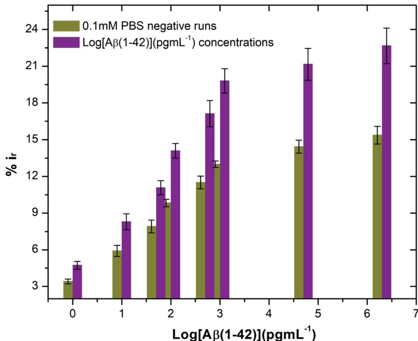
Fig. 5 Bar chart illustrating the peak current reduction (%*i*<sub>r</sub>) with exposure to 0.1 mM PBS only (negative runs with respect to each peptide concentration) and log of different concentrations of beta amyloid peptide Aβ(1-42) (*n* = 3).
