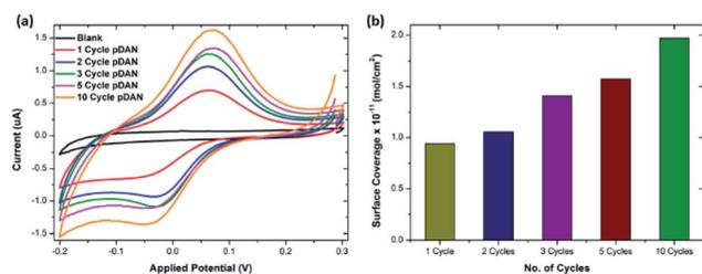
Fig. 1 (a) Cyclic voltammogram of ferrocene carboxylic acid functionalized SPGE and pDAN modified SPGEs at different scan cycles. PBS was used as the electrolyte and the CVs were recorded at a  $5 \text{ mV s}^{-1}$  scan rate. (b) Bar chart showing amine surface coverage vs. the number of pDAN scan cycles.
