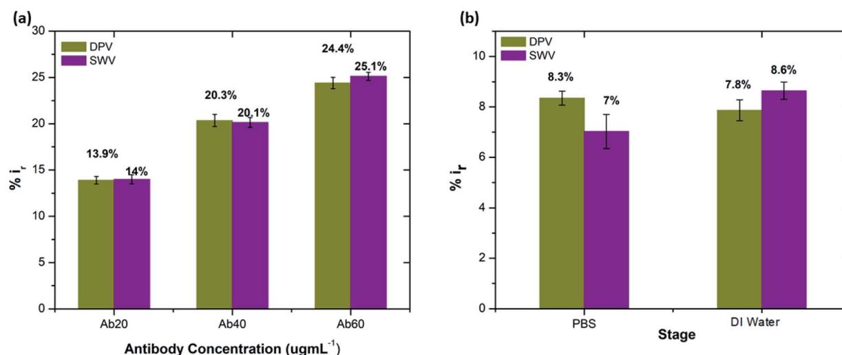
Fig. 4 (a) Peak current reduction in DPV and SWV measurements (% $i_r$ ) at each concentration of  $\text{A}\beta$  antibody. (b) Percentage reduction in peak current on exposure to DI water and PBS (0.1 mM) ( $n = 3$ ).
