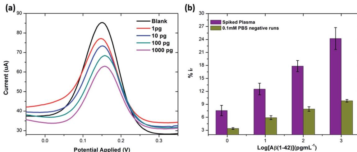
Fig. 8 (a) DPV response from spiked concentrations of Aβ(1-42) (at 1, 10, 100 and 1000 pg mL<sup>-1</sup>) in human plasma. (b) Bar chart illustrating the comparison of peak current reduction (%i<sub>r</sub>) with exposure to the different concentrations of Aβ(1-42) spiked in human plasma and 0.1 mM PBS (negative runs with respect to each peptide concentration) (n = 3).
