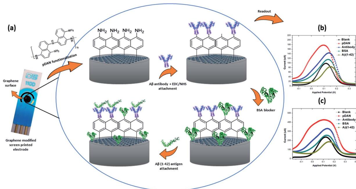
Fig. 3 (a) Schematic representation of the electrochemical immunosensor showing changes on the surface after each functionalization stage; (b) differential pulse voltammetry (DPV) response; (c) square wave voltammetry (SWV) response.
