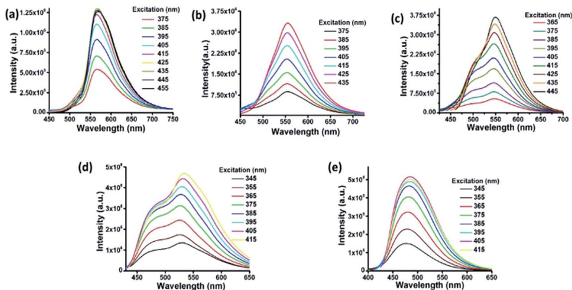
Fig. 2 Fluorescence spectra of C-dots2 (a) initially and after (b) 30 minutes, (c) 1 hour, (d) 1.5 hours and (e) 2 hours.
