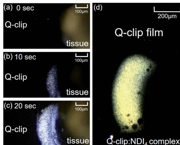
Fig. 5 *In situ* POM images documenting the adaptive assembly of the Q-clip : NDI<sub>4</sub> complex after addition of the saturated toluene solution of NDI from the tip of the tissue at (a) 0 s, (b) 10 s, and (c) 20 s. (d) The quick adaptive assembly of the Q-clip and NDI in the bulk phase.
