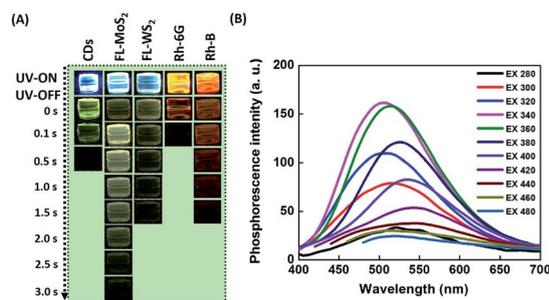
Fig. 2 Phosphorescence of nanomaterial- and organic dye-doped PVA composites. (A) Time-evolution photographs of PVA matrices incorporated with CDs, FL-MoS<sub>2</sub> QDs, FL-WS<sub>2</sub> QDs, Rhodamine 6G (Rh-6G), and Rhodamine B (Rh-B) before and after turning off a UV lamp (365 nm) at ambient temperature. (B) Phosphorescence spectra of the FL-MoS<sub>2</sub>/PVA composites as a function of excitation wavelength at ambient temperature.
