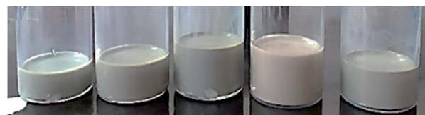
Fig. 1 AgNW ink sample of IPA : EG in a ratio of 85 : 15 with the AgNW concentration ranging from 10 \text{mg mL}^{-1} , 20 \text{mg mL}^{-1} , 30 \text{mg mL}^{-1} , 40 \text{mg mL}^{-1} to 50 \text{mg mL}^{-1} (left to right).
