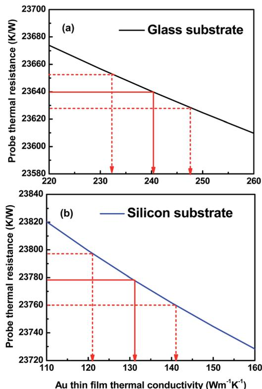
Fig. 6 3DFEM predictions of  $R_p^{\text{th}}$  vs. thermal conductivity of the thin film on (a) glass and (b) silicon substrates with 100 nm apex tip-sample clearance. Using the values of the experimental  $R_p^{\text{th}}$  the thermal conductivities and uncertainties of the thin films are determined by fitting, as shown by the red arrows.
