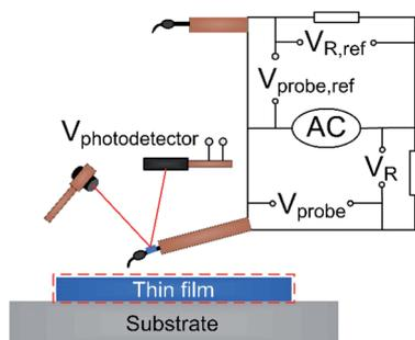
Fig. 2 Schematic of the non-contact SThM experimental setup. The voltage signal across the measurement probe ( $V_{\text{probe}}$ ), series resistor ( $V_{\text{R}}$ ), reference probe ( $V_{\text{probe,ref}}$ ), and reference series resistor ( $V_{\text{R,ref}}$ ) are recorded for thin-film thermal conductivity measurement. The voltage across the photodetector ( $V_{\text{photodetector}}$ ) is recorded to control the probe-sample clearance during the experiment.
