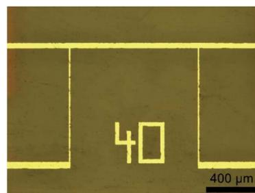
Fig. 1 Optical microscopy image of patterned Au thin film on silicon substrate.
