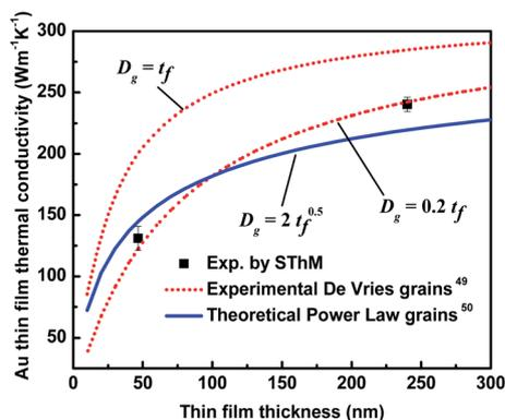
Fig. 8 Comparisons between the SThM experimental results (dots) and theoretical model predictions (lines) for thin film thermal conductivity based on ref. <sup>36</sup>. Theoretical predictions employ two grain size models, De Vries<sup>49</sup> and Power law.<sup>50</sup>
