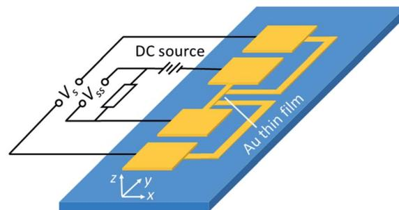
Fig. 7 Schematic of thin-film line instrumented for four-probe electrical resistance measurement. The voltage across the thin film line  $V_s$  and known series resistor  $V_{ss}$  yields the patterned line electrical resistance from which the thin film electrical resistivity is determined.
