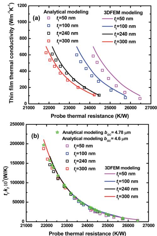
Fig. 10 Comparisons shown as a function of probe thermal resistance predicted from 3DFEM for films on glass substrate with  $t_f$  from 50–300 nm and  $k_f$  from 50–600  $\text{W m}^{-1} \text{ K}^{-1}$ : (a) between the actual  $k_f$  values used in the 3DFEM and the  $k_f$  obtained by fitting with analytical models; and (b) between the actual product of  $t_f$  with  $k_f$  and the product of  $t_f$  with  $k_f$  obtained by fitting with analytical models.
