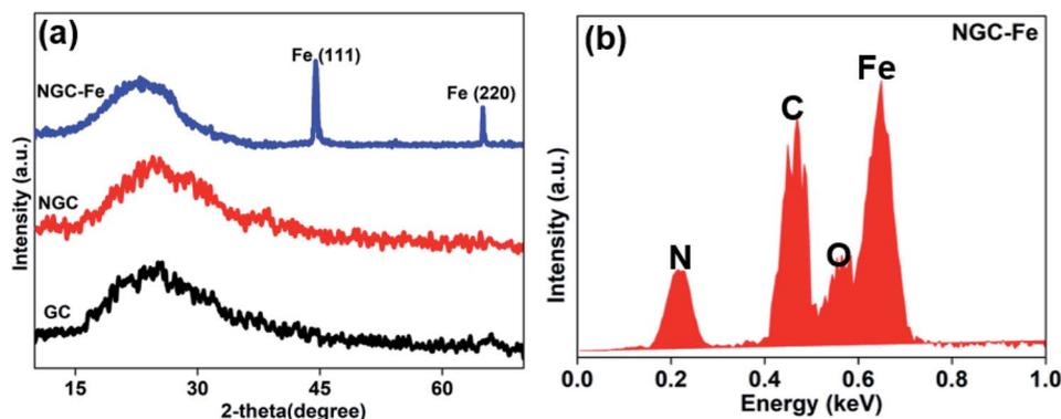
Fig. 1 (a) XRD patterns of GC, NGC and NGC-Fe samples; (b) EDS map of the NGC-Fe sample.
