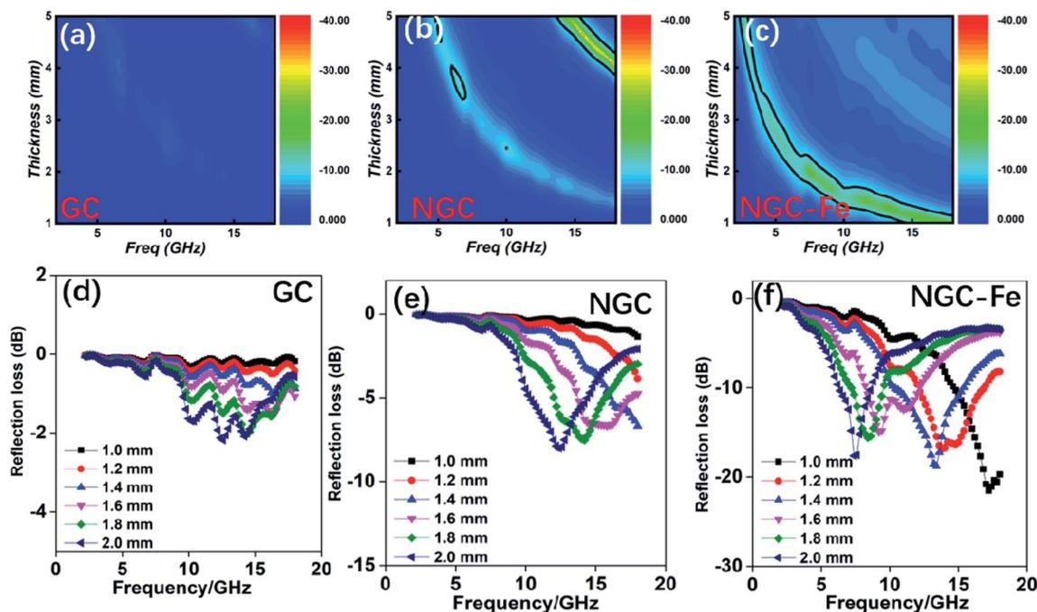
Fig. 6 Reflection loss values: (a and d) GC; (b and e) NGC; (c and f) NGC-Fe.
