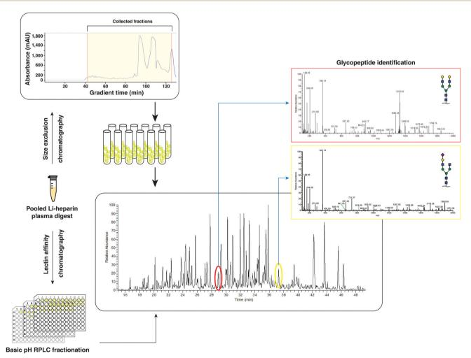
Fig. 1 N-Glycoproteomics workflow. A schematic workflow of size-exclusion chromatography, SEC-LC-MS/MS and lectin affinity chromatographybasic pH reversed phase liquid chromatography, LAC-bRPLC-LC-MS/MS that was employed is shown.
