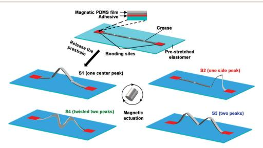
Fig. 1 Schematic illustration of the assembly and magnetic reconfiguration schemes of origami-inspired multistable ribbon structures.
