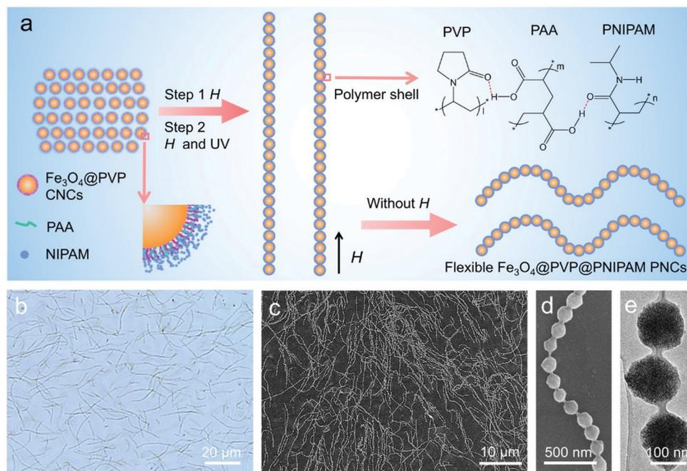
Fig. 1 The preparation and characterization of the typical  $\text{Fe}_3\text{O}_4@PVP@PNIPAM$  flexible PNCs. (a) Schematic illustration showing the formation process of the  $\text{Fe}_3\text{O}_4@PVP@PNIPAM$  flexible PNCs; (b) bright-field optical microscopy image; (c and d) SEM images; (e) TEM image.
