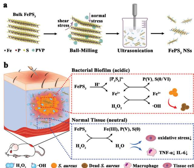
**Scheme 1** (a) Preparation of  $\text{FePS}_3$  NSs by ball-milling and ultrasonication method. (b)  $\text{FePS}_3$  NSs exhibit both self-enhanced Fenton activity in biofilm infected tissues with acidic pH for the eradication of biofilms and ROS scavenging properties in normal tissues with neutral pH for the remission of inflammation.
