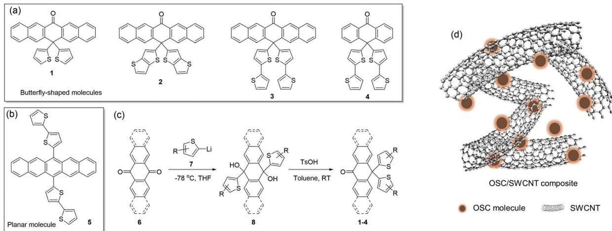
**Scheme 1** (a) Molecular structures of the studied butterfly-shaped OSCs **1–4**. (b) Molecular structure of the studied planar molecules **5**. (c) Synthesis of the butterfly-shaped OSCs **1–4**. (d) Illustration of the OSC/SWCNT composites.
