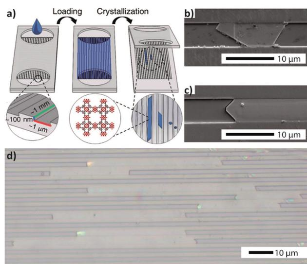
**Fig. 4** (a) Schematic illustration of the nanofluidic device used for the evaporation driven crystallization approach. (b and c) SEM images demonstrating the confined growth of HKUST-1 crystals in confined nano-chambers. (d) An optical image of high aspect ratio HKUST-1 crystals obtained *via* the method presented in (a). Reproduced with permission from ref. 42 published by The Royal Society of Chemistry.
