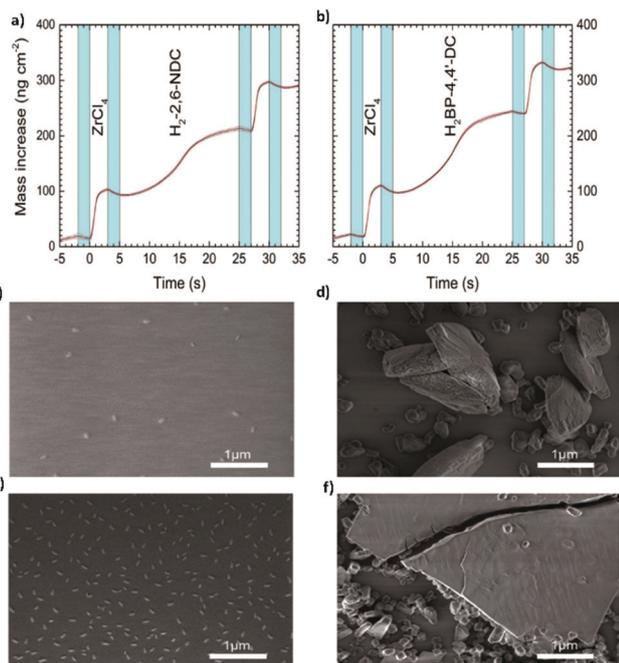
**Fig. 9** Mass increase during one MLD cycle (a) of the Zr-2,6-NDC process and (b) of the Zr-BP-4,4'-DC process, measured by the *in situ* QCM technique. (c) SEM picture of the as-deposited Zr-2,6-NDC film. (d) SEM picture of the Zr-2,6-NDC film after autoclave treatment. (e) SEM picture of the as-deposited Zr-BP-4,4'-DC film. (f) SEM picture of the Zr-BP-4,4'-DC film after autoclave treatment. Reproduced from ref. 11 with permission from The Royal Society of Chemistry.
