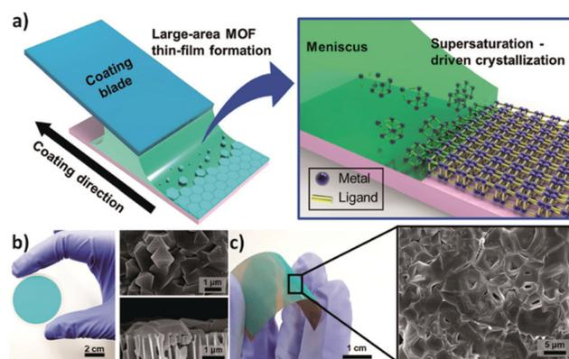
**Fig. 5** (a) Schematic representation of the meniscus-guided crystallization method and (b and c) optical and corresponding SEM images of HKUST-1 films coated onto different substrates, respectively on an AAO membrane and on a flexible polyimide film. Reproduced from ref. 44 with permission from American Chemical Society, copyright 2019.
