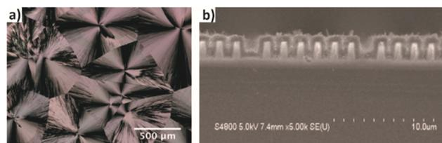
Fig. 7 (a) Optical microscope image of a film crystallized in moist air. (b) Cross-sectional FESEM image of a MOF-5 film deposited on a silicon substrate with trenches. Reproduced from ref. 58, copyright (2013), with permission from Elsevier.
