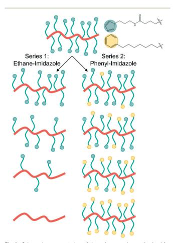
Fig. 1 Schematic representation of the polymer series synthesized for this study. Series 1 changes the imidazole grafting density by replacing imidazole with a non-bulky ethane inert side chain, while series 2 replaces the imidazole with a phenyl inert side chain to maintain similar steric bulk.
