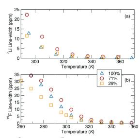
Fig. 7 (a)  $^{7}$ Li NMR and (b)  $^{19}$ F NMR peak width, as a function of temperature. All samples consist of a 0.1 Li:monomer ratio of LiTFSI added to the polymer.
