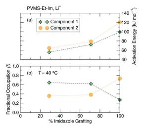
Fig. 8 (a) Activation energies and (b) fractional occupation at 40 °C of the two Li<sup>+</sup> components as a function of imidazole grafting density, extracted from  $^{7}$ Li  $T_{1\rho}$  measurements as a function of temperature. Lower grafting density results in higher mobility and occupation of the more mobile Li environment. All samples consist of a 0.1 Li: monomer ratio of LiTFSI added to the polymer.
