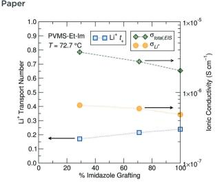
Fig. 6 Transport numbers (Li $^+$   $t_+$ ), total EIS-measured ionic conductivity ( $\sigma_{\text{total,EIS}}$ ) and adjusted Li $^+$ -ion conductivity ( $\sigma_{\text{Li}^+}$ ) for the three PVMS-Et-Im grafting density polymers measured using PFG-NMR at 72.7 °C. All samples consist of a 0.1 Li:monomer ratio of LiTFSI added to the polymer.
