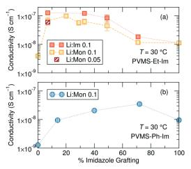
Fig. 4 Total ionic conductivity for the (a) ethane-imidazole and (b) phenyl-imidazole series as a function of the percentage of monomers containing an imidazole sidechain.
