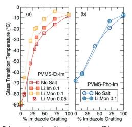
Fig. 3 Polymer glass transition temperature  $(T_q)$  versus grafting density for the (a) ethane-imidazole and (b) phenyl-imidazole polymer grafting series. A lower imidazole content results in lower  $T_{\rm q}$  due to the removal of the polar and hydrogen-bonding groups. The lower steric bulk of the ethane side chain results in a lower  $T_{\alpha}$  (-90 °C) than the fully phenyl-functionalized polymer (-68 °C).
