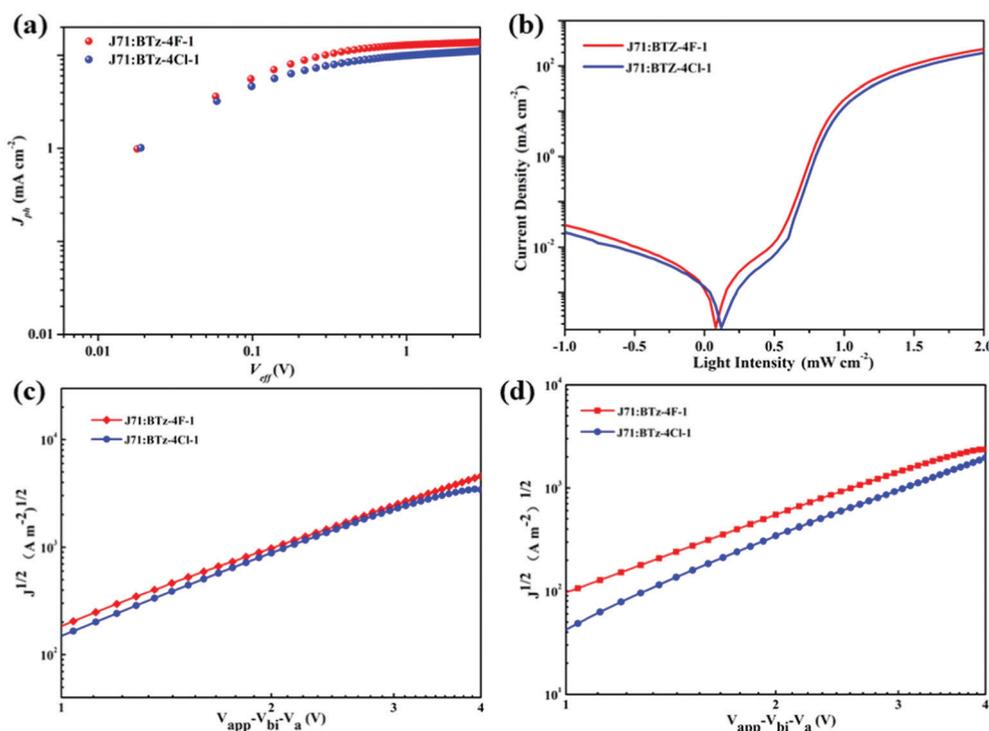
**Fig. 6** (a)  $J_{ph}$ - $V_{eff}$  and (b) dark current density curves of J71: BTz-4F-1 and J71: BTz-4Cl-1 blend OSCs under optimal conditions;  $J^{1/2}$ - $V$  plots of the hole-only devices (c) and the electron-only devices (d) based on the J71: BTz-4F-1 and J71: BTz-4Cl-1 blends.
