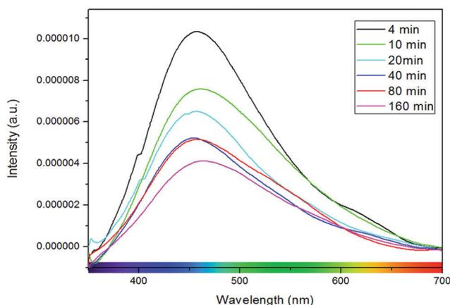
**Fig. 14** Photoluminescence spectra of STO nanoparticles with different synthesis times. Longer synthesis times correspond to larger particles and to lower photoluminescence intensities. Reprinted with permission from ref. 114. Copyright 2012 American Chemical Society.
