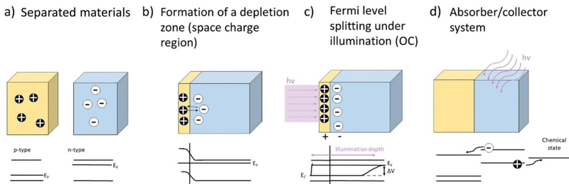
Fig. 16 Schematic representation of the generation of a photovoltage at a heterojunction. A p-type and an n-type material are brought into contact (a), forming a space charge region with a built-in field (b). Under UV illumination and generation of electron/hole pairs, a splitting of the Fermi level occurs under open circuit conditions (c). Absorber/collector systems use semiconductors or Red-Ox systems to separate generated charge carriers in the resulting energy landscape (d).
