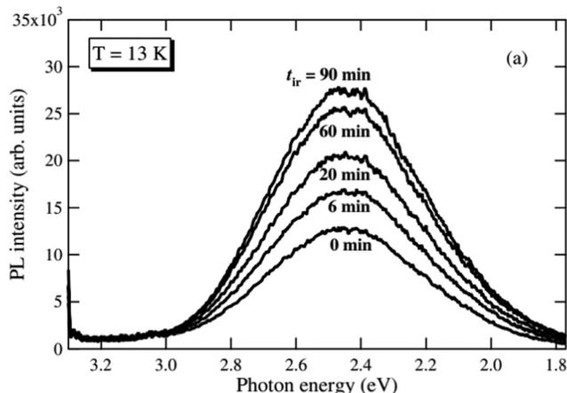
Fig. 11 Photoluminescence spectra recorded at 13 K after different annealing times in vacuum under 325 nm laser light irradiation.<sup>97</sup> Reprinted by permission from IOP Publishing (2005).
