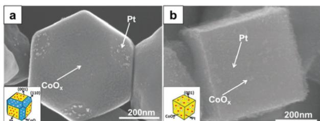
Fig. 27 (a) 18-Facet STO crystal with spatially separated Pt and  $\text{CoO}_x$  cocatalysts. (b) Cubic STO with only {001} facets present and cocatalysts distributed randomly. Reprinted from ref. 358, with permission from the Royal Society of Chemistry.
