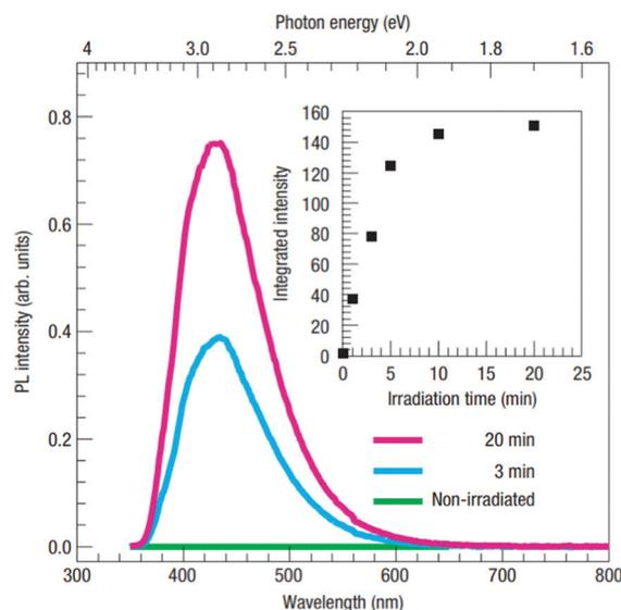
Fig. 13 Photoluminescence spectra of Ar<sup>+</sup> irradiated STO measured for different irradiation times at room temperature. The inset shows the intensity increasing with irradiation time.<sup>103</sup> Reprinted by permission from Nature materials (2005).
