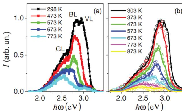
**Fig. 15** Photoluminescence spectrum with three separate luminescence bands (green – GL, blue – BL and violet – VL) of undoped STO at excitation energies of 2.2 mJ cm<sup>-2</sup> (a) and 22 mJ cm<sup>-2</sup> (b), recorded at temperatures between 298 and 873 K. Reprinted from ref. 111, with the permission of AIP Publishing.
