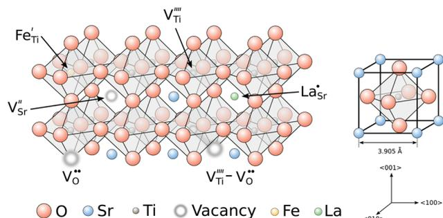
Fig. 1 Schematic structure of strontium titanate with different defects integrated in the lattice. All defect species are written according to the Kröger–Vink notation.<sup>49</sup>
