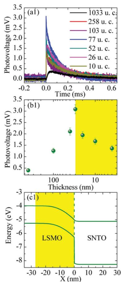
Fig. 18 (a and b) Thickness dependence of the photovoltage developing at the junction of a La<sub>0.9</sub>Sr<sub>0.1</sub>MnO<sub>3</sub> thin film on Nb doped SrTiO<sub>3</sub> (energy landscape shown in (c)). A maximum is found for approximately 30 nm which is the width of the depletion region. Reprinted from ref. 161, with the permission of AIP Publishing.
