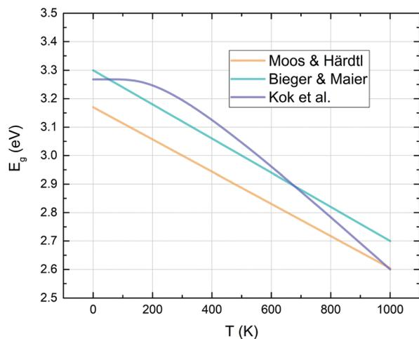
Fig. 2 Indirect band gap energies of strontium titanate – curves calculated with the fit formulae proposed by different authors.<sup>34,54,55</sup>
