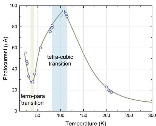
Fig. 4 Photocurrent in STO as a function of temperature. Applied potential was 22.5 V and the measured dark currents were  $1.2 \times 10^{-12}$  A at 300 K and less than  $10^{-14}$  A at 77 K. Reprinted from ref. 69, with the permission of AIP Publishing.
