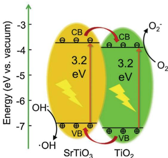
Fig. 24 STO and TiO<sub>2</sub> based type II hetero junction to illustrate the band positions and mechanisms responsible for the photocatalytic activity. Reprinted from ref. 242, with permission from Elsevier.
