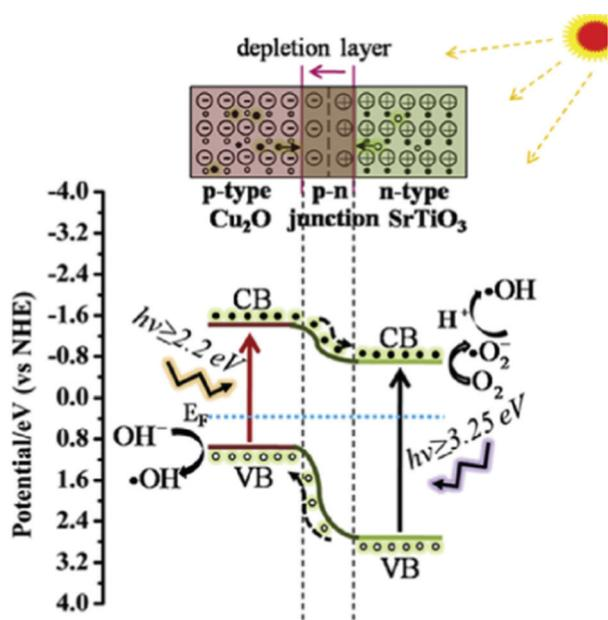
Fig. 25 Schematic illustration of the n-STO/p-Cu<sub>2</sub>O p-n junction, with a built-in internal electric field, helping to separate charge carriers, thus suppressing recombination. Reprinted from ref. 334, with permission from Elsevier.
