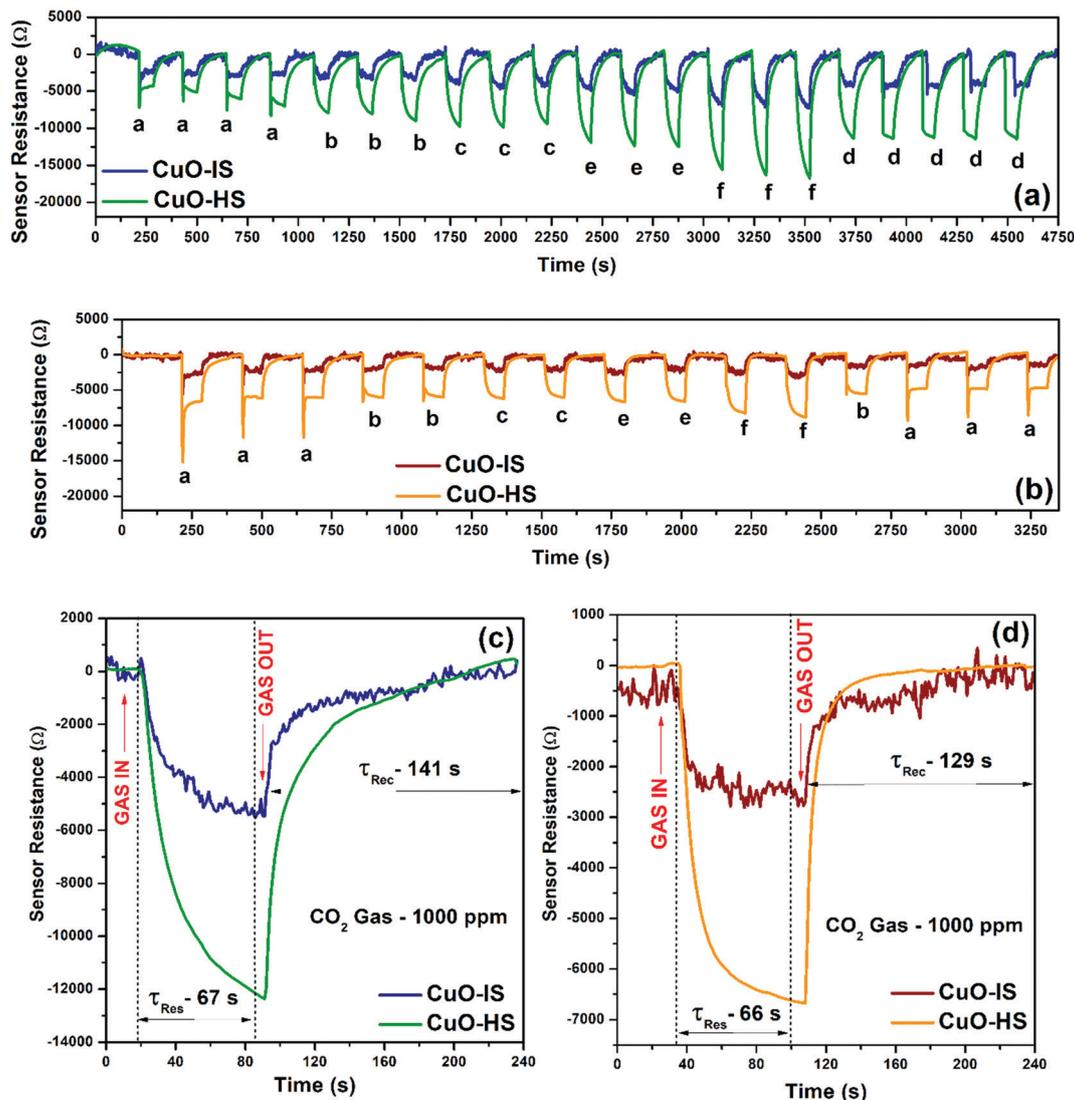
Fig. 5 Dynamic transients as a function of gas concentrations measured in (a) dry air and (b) humid conditions. Response kinetics measured in (c) dry air and (b) humid air. All the  $\text{CO}_2$  sensor characteristics were studied at room temperature (that is,  $32^\circ\text{C}$ ). Wet conditions refer to 59% relative humidity measured at  $32^\circ\text{C}$ .
