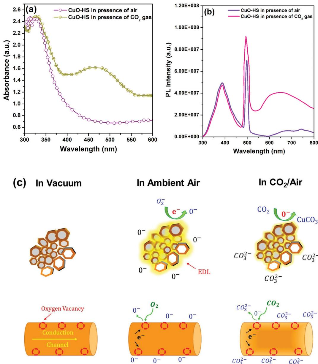
Fig. 7 *In situ* measurements for the identification of oxygen vacancies (a) UV diffuse reflectance spectra, (b) photoluminescence spectra achieved in the presence of air and CO<sub>2</sub> gas, and (c) schematic illustration depicting the CO<sub>2</sub> sensing phenomenon at room temperature over hexagonal CuO sheets.
