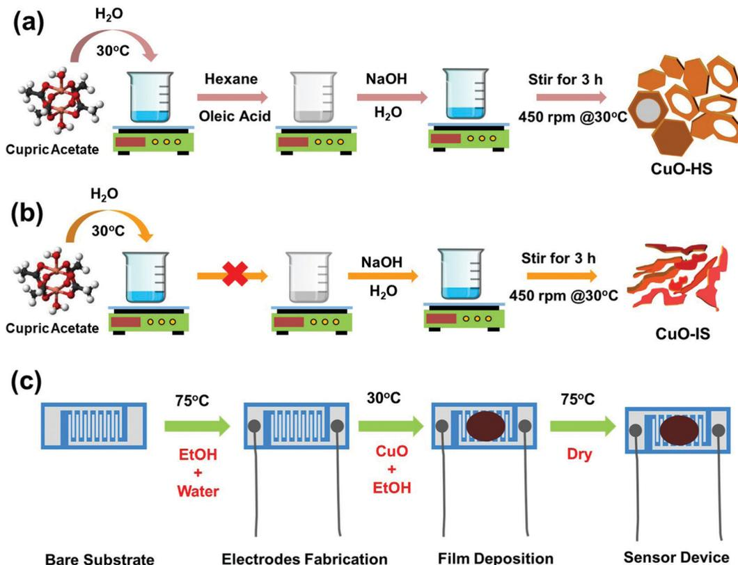
Fig. 1 Schematic representation illustrating methodologies followed to achieve (a) solid/hollow hexagonal sheets (CuO-HS) and (b) irregular sheets (CuO-IS). (c) Fabrication of sensor device for CO<sub>2</sub> gas monitoring.
