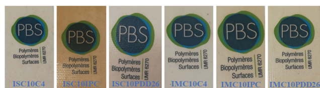
Fig. 1 Copolyester films prepared by hot pressing.
