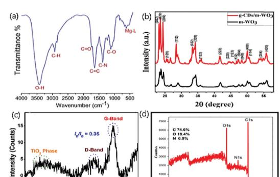
Fig. 3 (a) FT-IR spectra of red emitting Mg-N-CDs; reproduced with permission from ref. 55 Copyright 2018 American Chemical Society. (b) XRD pattern of bare WO<sub>3</sub> and CDs/WO<sub>3</sub>; reproduced with permission from ref. 71 Copyright 2020 Elsevier. (c) Raman spectra of TiO<sub>2</sub>/CDs; reproduced with permission from ref. 66 Copyright 2018 Elsevier. (d) XPS spectrum of N/CDs; reproduced with permission from ref. 43 Copyright 2018 Elsevier.
