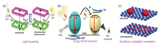
Fig. 5 Systematic representation of (a) light-harvesting (b) charge transfer dynamics (c) surface catalytic reaction.
