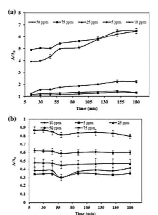
Fig. 7 Effect of initial concentration on photocatalytic degradation of (a) CR dye and (b) MB dye; reproduced with permission from ref. 137 Copyright 2020 Springer.
