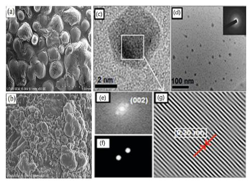
Fig. 1 SEM images of (a) N/CQDs at 50× magnification (b) CQDs at 500× magnification; reproduced with permission from ref. 67 Copyright 2021 Elsevier; (c) HRTEM of reduced CDs; (d) particle distribution of reduced CDs (inset: SAED image); FFT of reduced CDs (e) before & (f) after masking; (g) IFFT of reduced CDs exhibiting lattice fringes; reproduced with permission from ref. 44 Copyright 2017 American Chemical Society.
