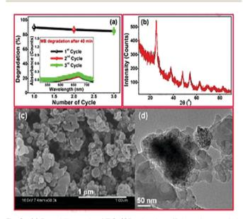
Fig. 9 (a) Reusability study of TiO<sub>2</sub>/CDs showing efficient photocatalytic activity for 3 cycles; stability study by employing characterization such as (b) XRD spectrum; (c) FESEM and (d) TEM; reproduced with permission from ref. 66 Copyright 2018 Elsevier.
