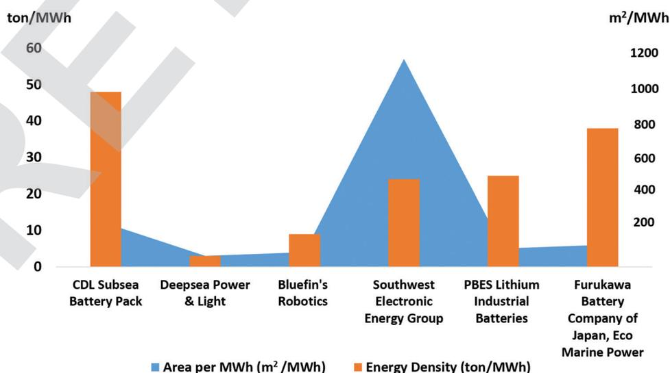
Fig. 2 Comparison of various marine batteries.
