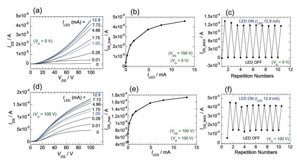
Fig. 7 (a)  $I_{DS}$  plots for FET **2** depending on  $I_{LED}$  (at  $V_G = 0$  V). (b)  $I_{DS}$  maxima of FET **2** with respect to  $I_{LED}$ , (at  $V_G = 0$  V, and  $V_{DS} = 100$  V). (c) Changes in  $I_{DS}$  values of FET **2** at  $V_G = 0$  V, when LED is switched on and off, repeatedly. (d–f) Similar experimental plots performed at  $V_G$  100 V.
