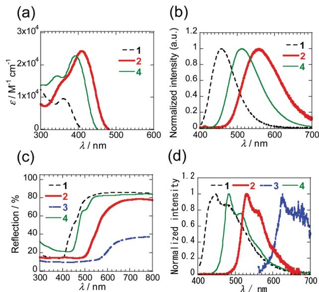
Fig. 4 (a) UV-Vis (<10<sup>-5</sup> M) and (b) PL spectra of **1**, **2** and **4** in DCM. The spectra of **3** with low solubility are shown in Fig. S3 and S4 (ESI<sup>†</sup>). (c) Solid diffuse reflection spectra of **1–4**. (d) PL spectra of **1–4** in solid states.
