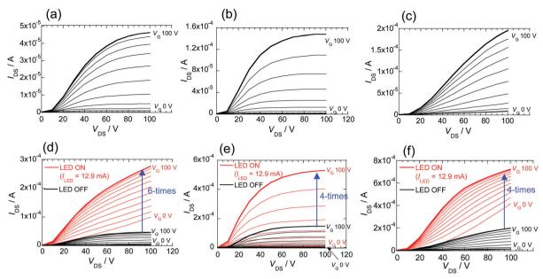
Fig. 6 FET characteristics of (a) biselenophene derivative 2, (b) terselenophene derivative 3, and (c) phenylselenophene derivative 4 under dark conditions. FET characteristics of (d) 2, (e) 3, and (f) 4 during photoirradiation (bold red lines). Solid black lines are output curves under dark conditions.
