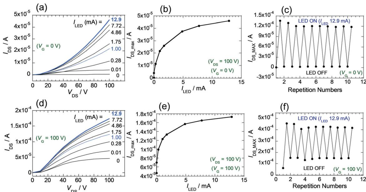
Fig. 7 (a)  $I_{DS}$  plots for FET **2** depending on  $I_{LED}$  (at  $V_G = 0$  V). (b)  $I_{DS}$  maxima of FET **2** with respect to  $I_{LED}$ , (at  $V_G = 0$  V, and  $V_{DS} = 100$  V). (c) Changes in  $I_{DS}$  values of FET **2** at  $V_G = 0$  V, when LED is switched on and off, repeatedly. (d–f) Similar experimental plots performed at  $V_G = 100$  V.
