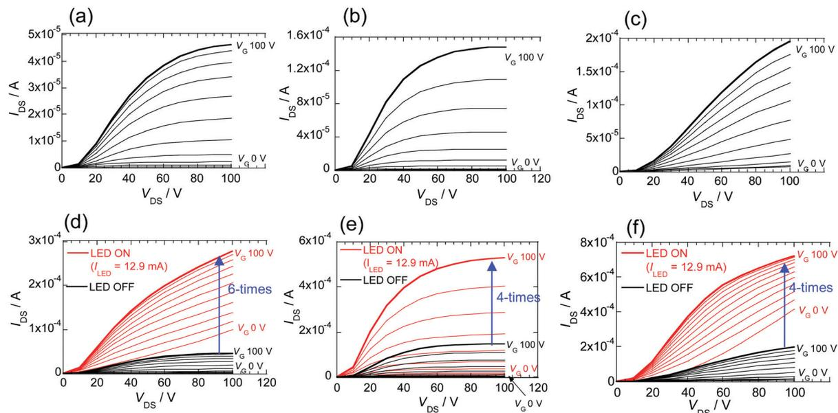
Fig. 6 FET characteristics of (a) biselenophene derivative **2**, (b) terselenophene derivative **3**, and (c) phenylselenophene derivative **4** under dark conditions. FET characteristics of (d) **2**, (e) **3**, and (f) **4** during photoirradiation (bold red lines). Solid black lines are output curves under dark conditions.
